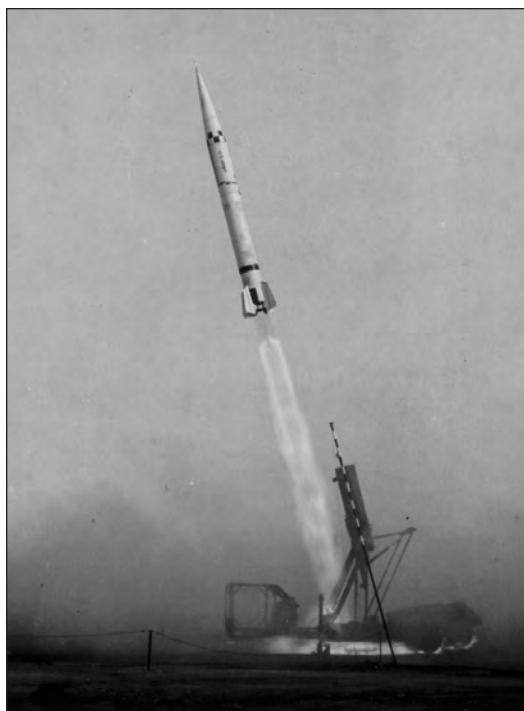
Sergeant, an inertially guided, solid-propellant, surface-to-surface, ballistic missile launches from White Sands missile range in the course of JPL's four-year development and production program for the U.S. Army, 1956-1960 (Photo: NASA/JPL-Caltech Archives, Photo number 293-3302B).
