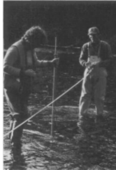
Boh Erhardt (left) and an assistant assess stream profile on the Kadashan River, Chichagof Island. (Swanston collection)
