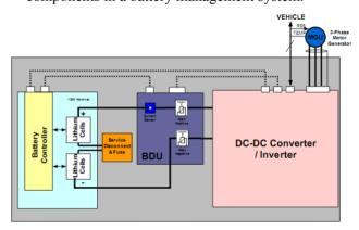
Figure 3: Electrical components of a battery pack, from [3]
