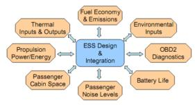
Figure 2: Components in battery pack integration and interface with vehicle, adapted from [1]
