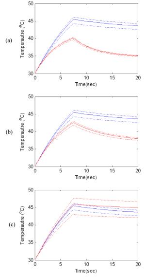
Figure 6: (a) Comparison of average temperatures (solid line) and maximum/minimum temperatures (dotted) time variation for Cell AP (blue) and Cell BP (red) with midsize PHEV10 US06 driving scenario; (b) same for Cell AP (blue) and Cell CP (red); (c) same for Cell AP with different layer normal conductivity, 0.8 W/mK (blue) and 0.2 W/mK (red)
