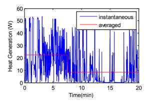
Figure 5: Instantaneous and averaged heat generation rate per cell (20 Ah)
