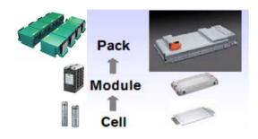
Figure 1: Cell, module, and pack
