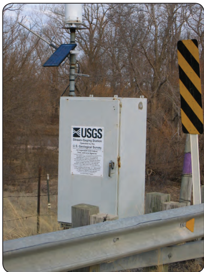
U.S. Geological Survey streamflow-gaging station. Photograph by Jennifer Graham, U.S. Geological Survey.
