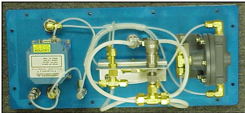
Figure 6: Back View of Pressure Control Unit
