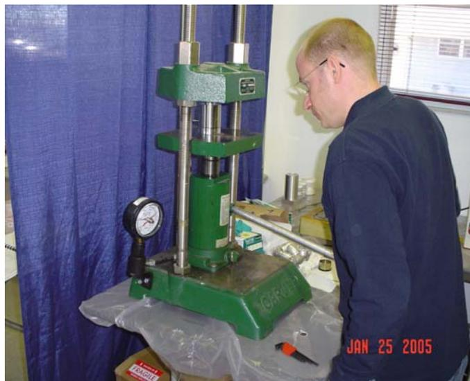
**Figure 6-2. Oxford ED2000 soil pellet sample preparation.**
