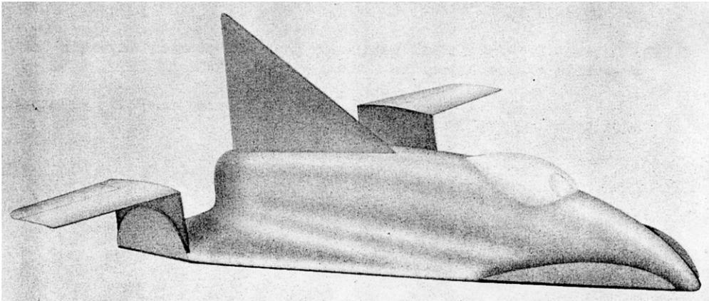
from others in the Aircraft Loads Branch and the Performance Branch, made detailed studies of such aspects as heating, structural loads, and stability and control. The vehicle was sized to weigh about 2000 pounds, the same as the Mercury capsule, so that it could be carried on the nose of the Atlas Rocket. Preliminary calculations showed that a vehicle capable of carrying a single astronaut could be made within this weight limitation.
