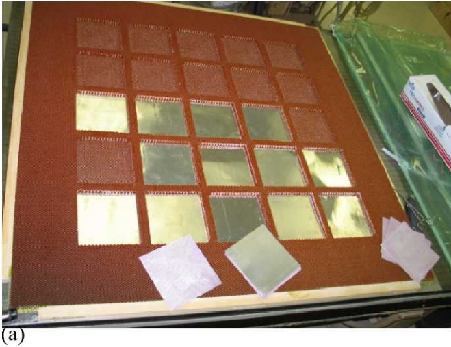
Fig. 22 Reinforced recessed core with 25 6" recesses, 0.5" deep (a), transmission loss (b) and band average difference in TL, (c).
