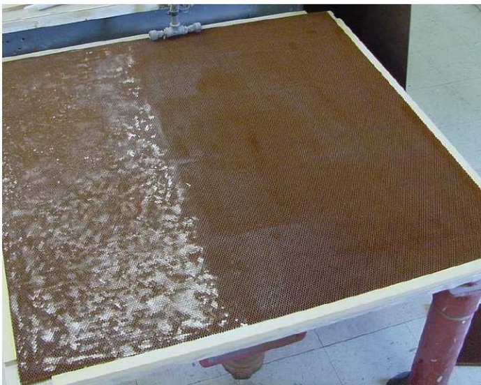
Fig. 37 NASA panel with Perlite treatment about 40% complete.
