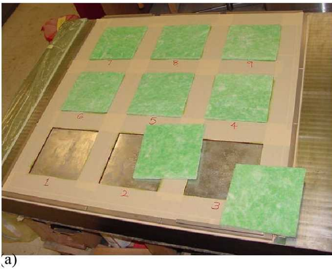
Fig. 23 Reinforced recessed core with 10 inch squares, fiberglass filled (a), wavenumber spectrum (b).
