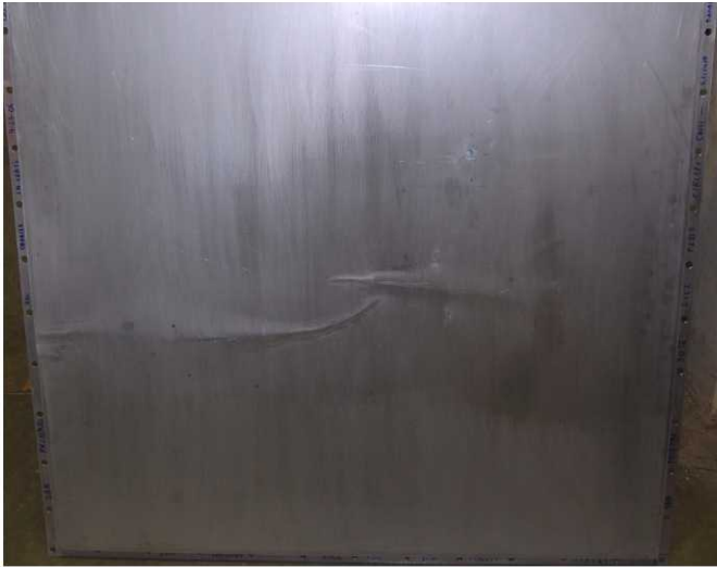
Fig. 38 Rocketdyne panel with 30% Perlite fill. Area of unbonded face sheet detailed.
