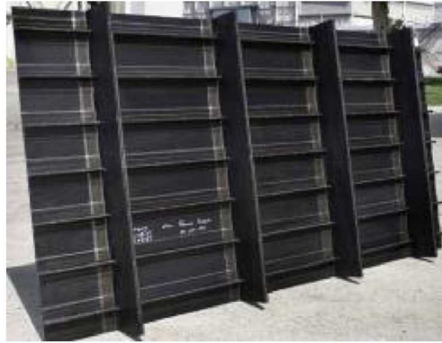
Figure 1. Cured panel prior to extraction of test specimens.
