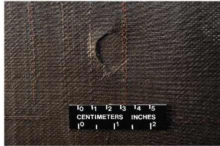
Figure 7. Machining damage to specimen F4.
