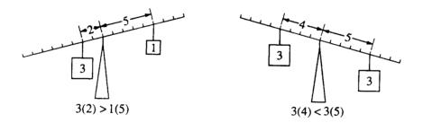
(A) Draw two 9-pound weights attached to the beam so that the beam will be in balance. Label the 9-pound weights and their distance from the pivot.
