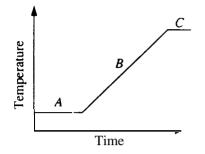
A beaker contains a mixture of water and ice. A thermometer is placed in this mixture, and the mixture is continuously stirred as it is heated to boiling over a flame. At regular intervals, the temperature of the mixture is recorded. These data are then used to produce the graph above. In the space provided below, briefly explain the appearance of each labelled section of the curve.
