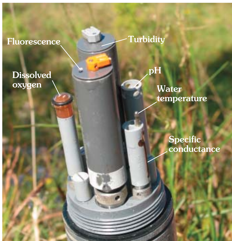
Figure 2. Multiparameter monitor used to measure turbidity, specific conductance, pH, water temperature, dissolved oxygen, and fluorescence in water during sample collection and for in-stream continuous monitoring.
