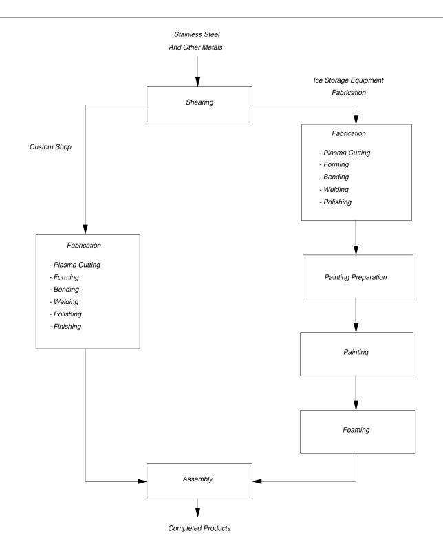
Figure 1. Abbreviated process flow diagram for production of food service equipment.
