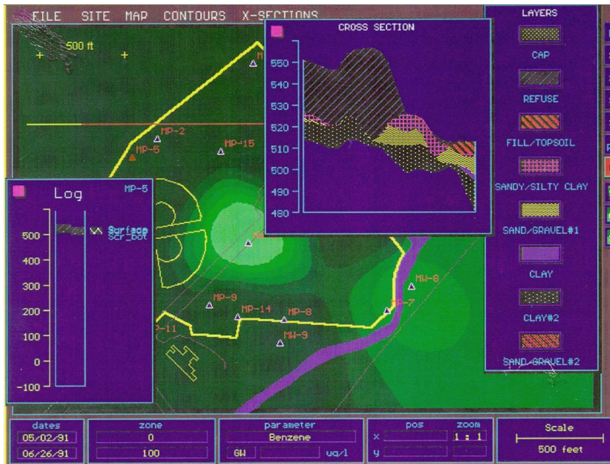
Figure 6. GEOS computer screen showing organic contaminant plume in relation to subsurface stratigraphy (see text for discussion).
