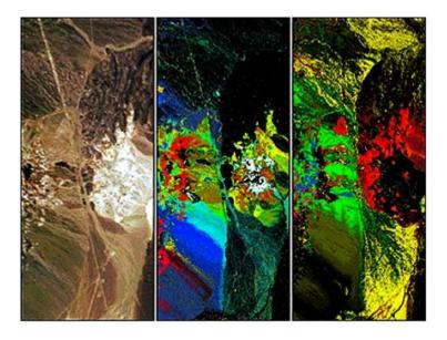
Figure 4: Comparison of Two False-Color HSI Images with Natural Color Photo<sup>13</sup>
