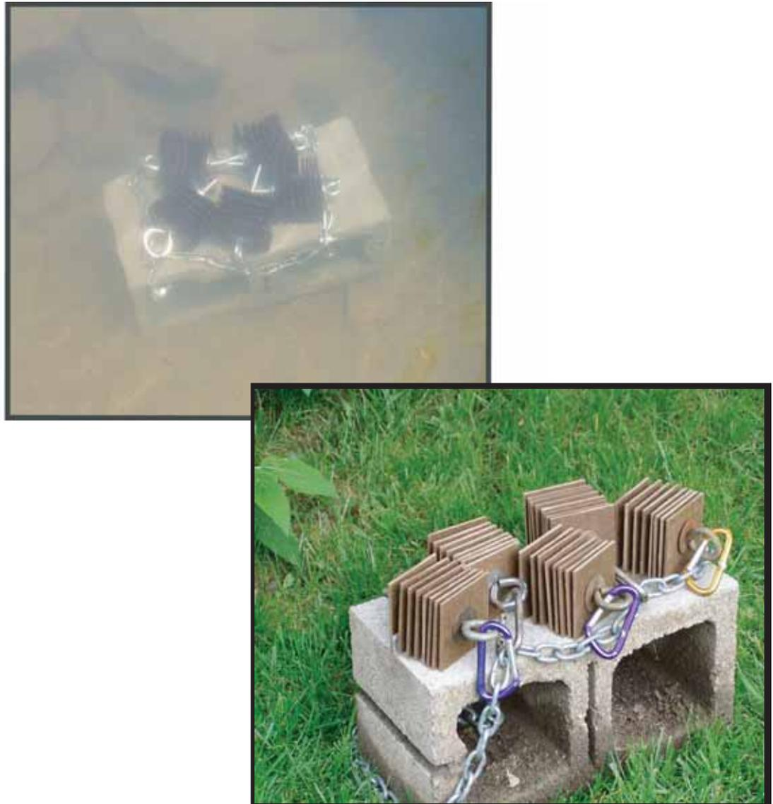
**Figure 3.** Modified Hester-Dendy samplers used to collect artificial-substrate samples. The top photograph shows one of the two sampling units placed in Nineveh Creek at site B2 on June 17, 2002, U.S. Army Atterbury Reserve Forces Training Area, near Edinburgh, Indiana. The bottom photograph shows a plate-type artificial-substrate sampler on dry land before being placed in the stream.
