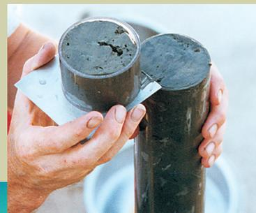
Slicing a 5-centimeter long subsample from a core for laboratory analysis.
