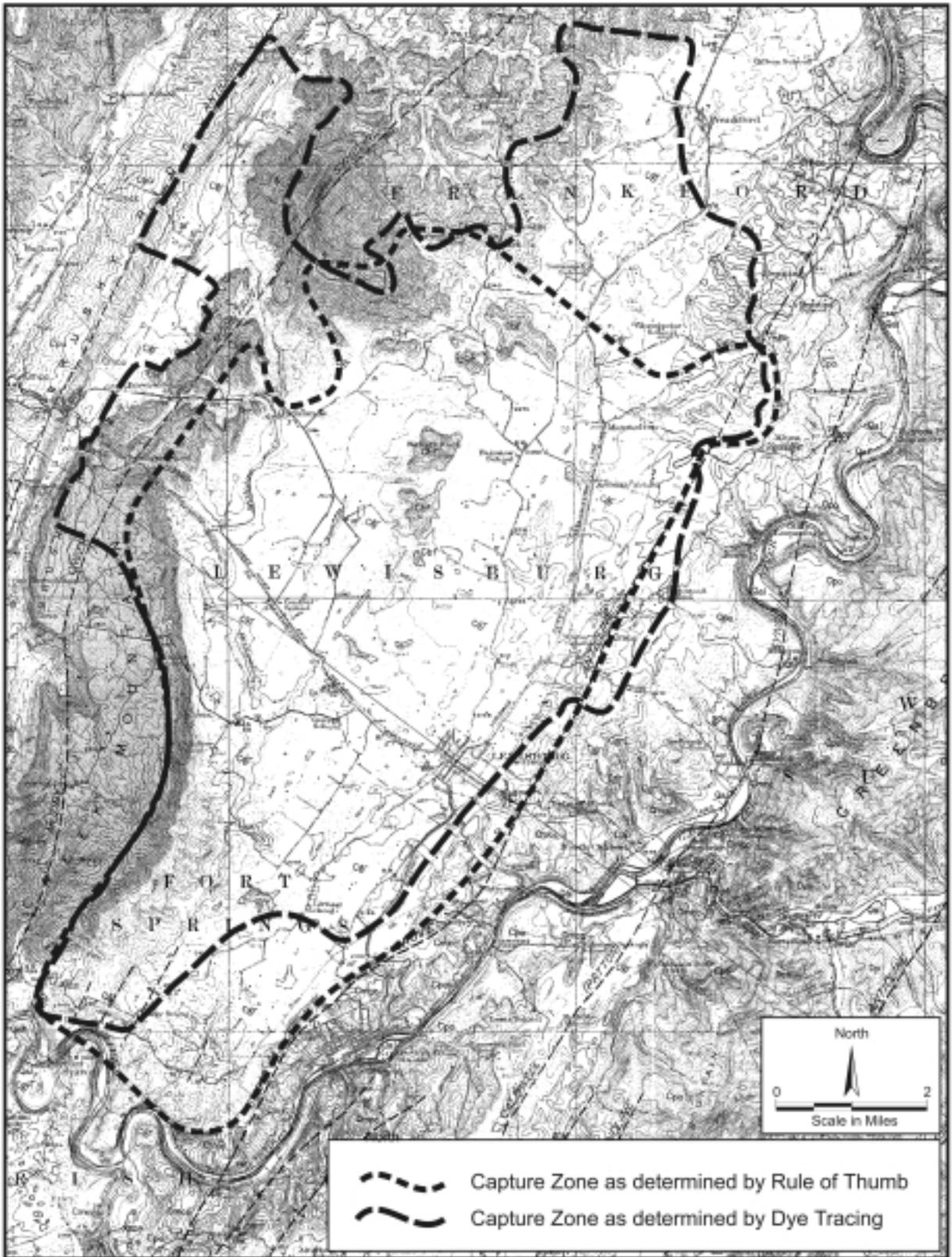
Figure 9. Davis Spring, Greenbrier County, West Virginia. The capture zone estimated with RT 1.1 is shown superimposed on the capture zone estimated by Jones (1997) on the basis of dye tracing. (The strike line extending from Davis Spring follows the axis of a syncline, and so the updip projection is made in both directions away from the strike line.)
