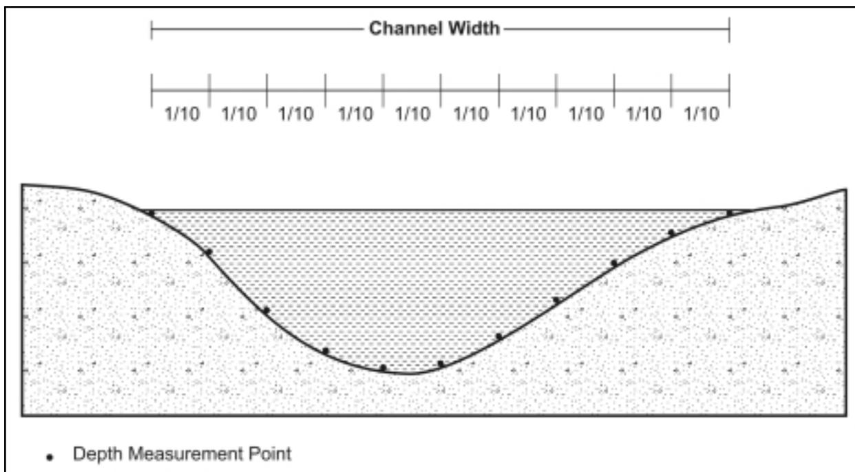
Figure 17: Cross section of a stream, with locations of depth-measurement points.
