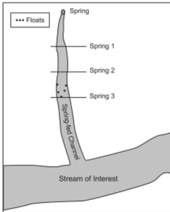
Figure 16: b) Position of floats at the end of a stream-velocity measurement.
