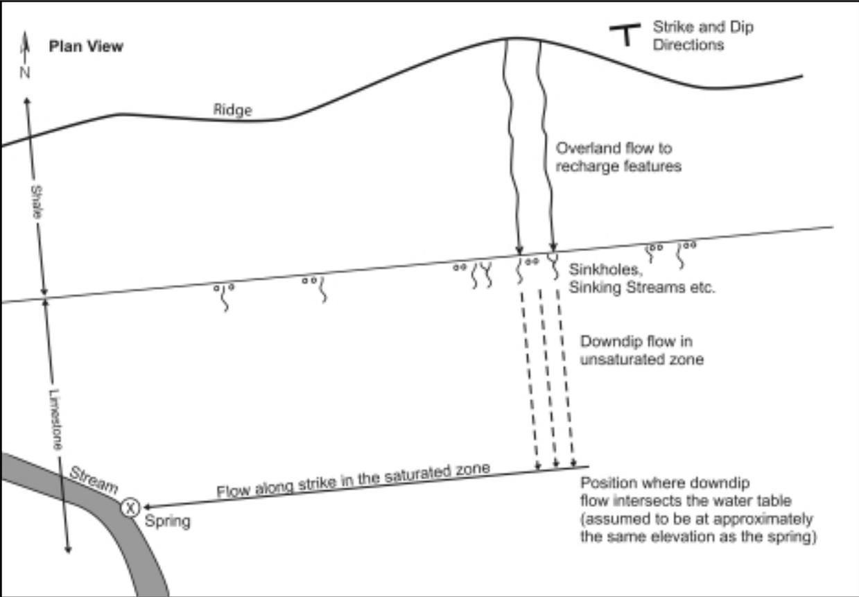
Figure 2. Generalized karst ground-water flow in the Appalachians.
