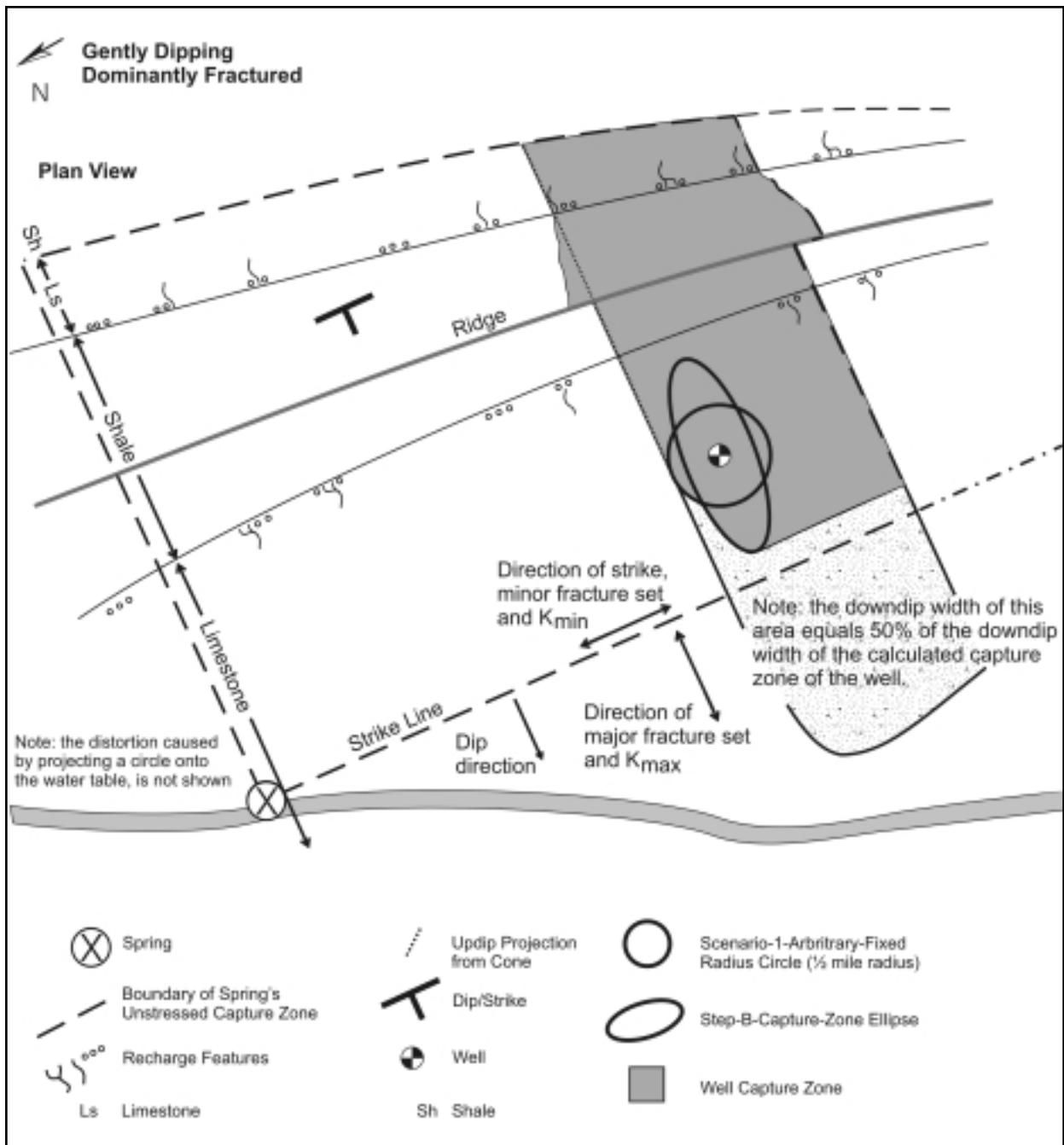
Figure 14. Capture zone of a well, located far enough from the headward boundary of the spring's capture zone that there is no interference, in a gently dipping, dominantly fractured aquifer.
