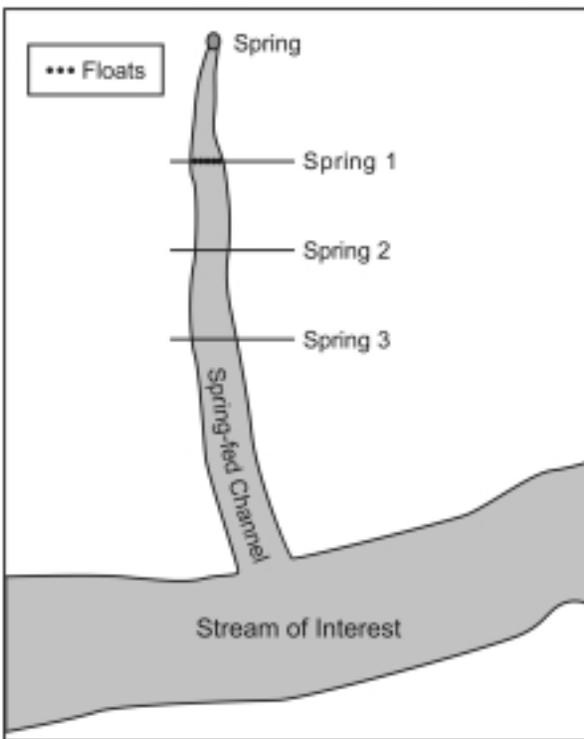
Figure 16: a) Position of floats at the beginning of a stream-velocity measurement.
