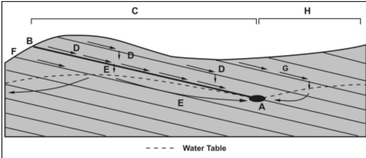
Figure 15. Cross section through a typical capture zone, showing the basic premise behind the Rules of Thumb. (View is in the direction of the strike, that is, strike is into/out of the page.)
