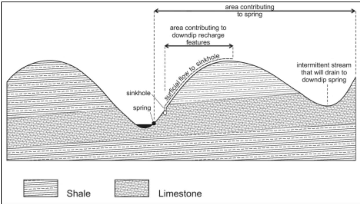
Figure 6. Cross section view of a spring capture zone where the updip projection of the karst aquifer extends beyond the ridge, and the updip valley is flooded by carbonate rock.
