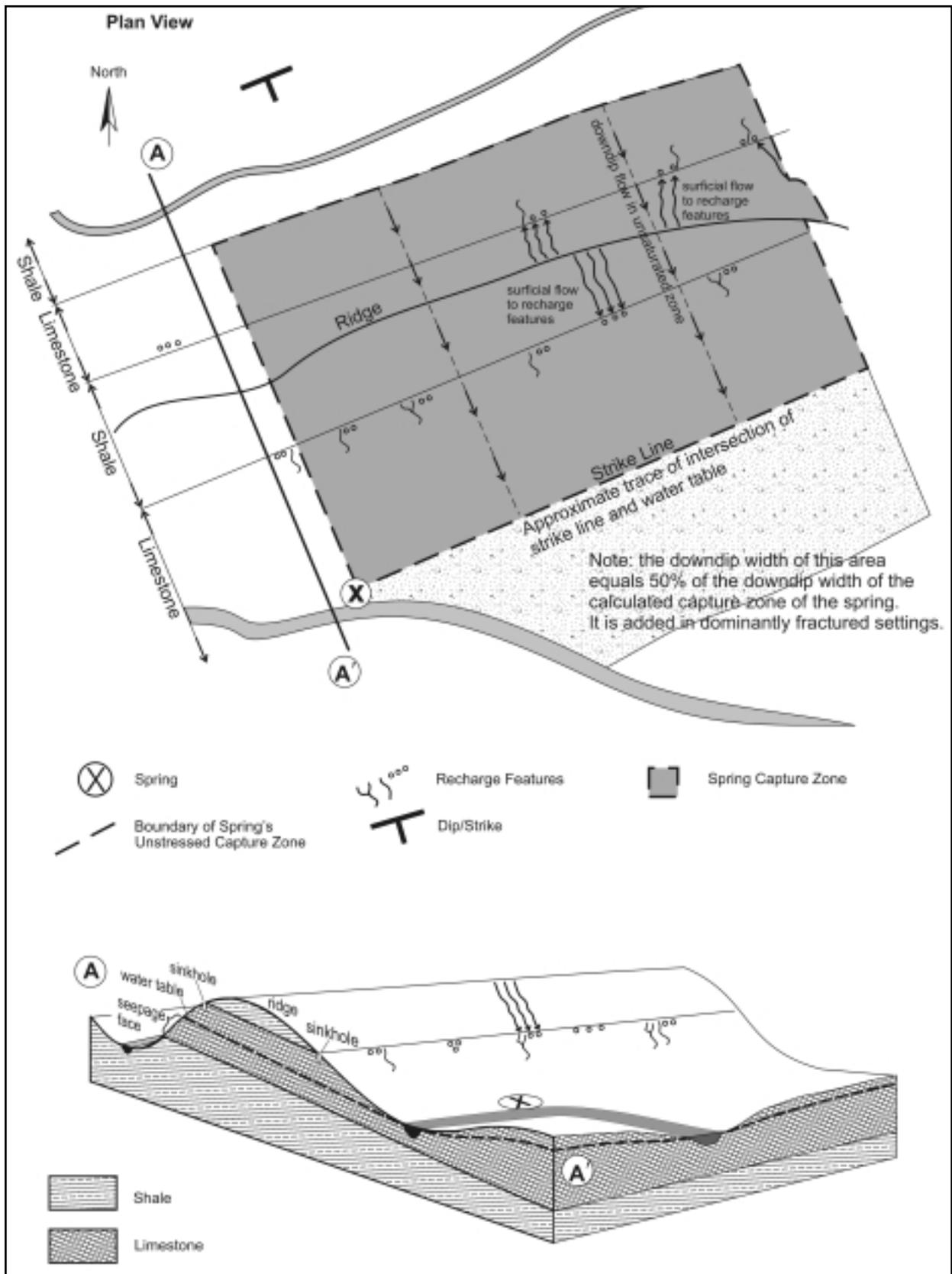
Figure 5. Spring capture zone in plan and three-dimensional views.
