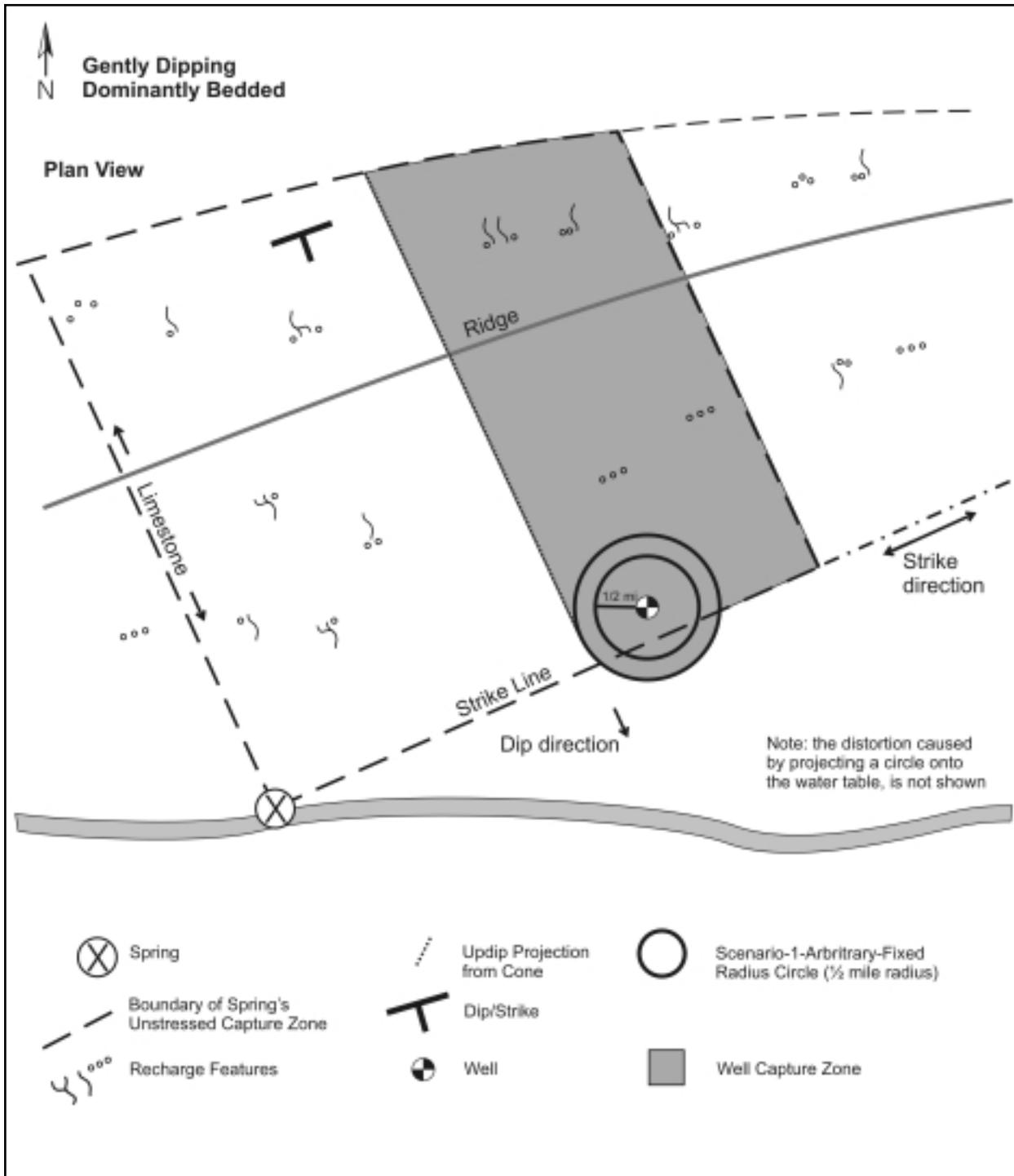
Figure 13. Capture zone of a well, located far enough from the headward boundary of the spring's capture zone that there is no interference, in a gently dipping, dominantly bedded aquifer.
