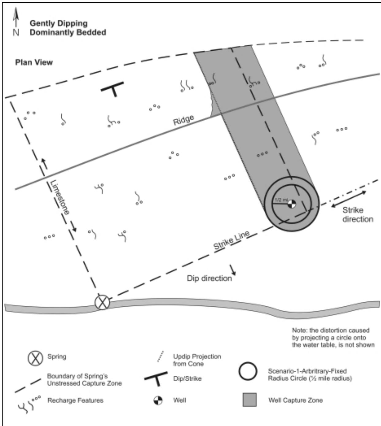
Figure 12. Capture zone of a well, located near the headward boundary of the spring's capture zone, in a gently dipping, dominantly bedded aquifer.
