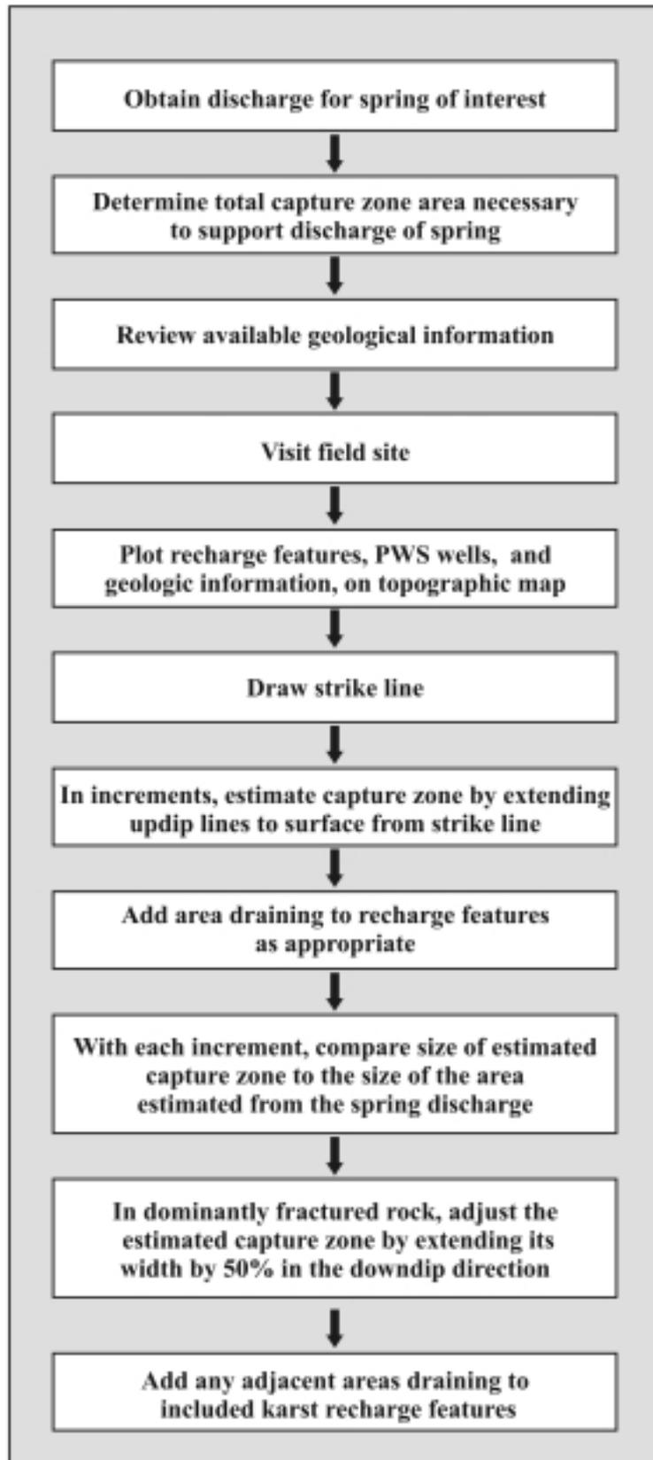
Figure 4. Flowchart for general Rules-of-Thumb process for estimating the capture zones for karst springs and wells in the Ridge and Valley and Appalachian Plateaus Provinces.
