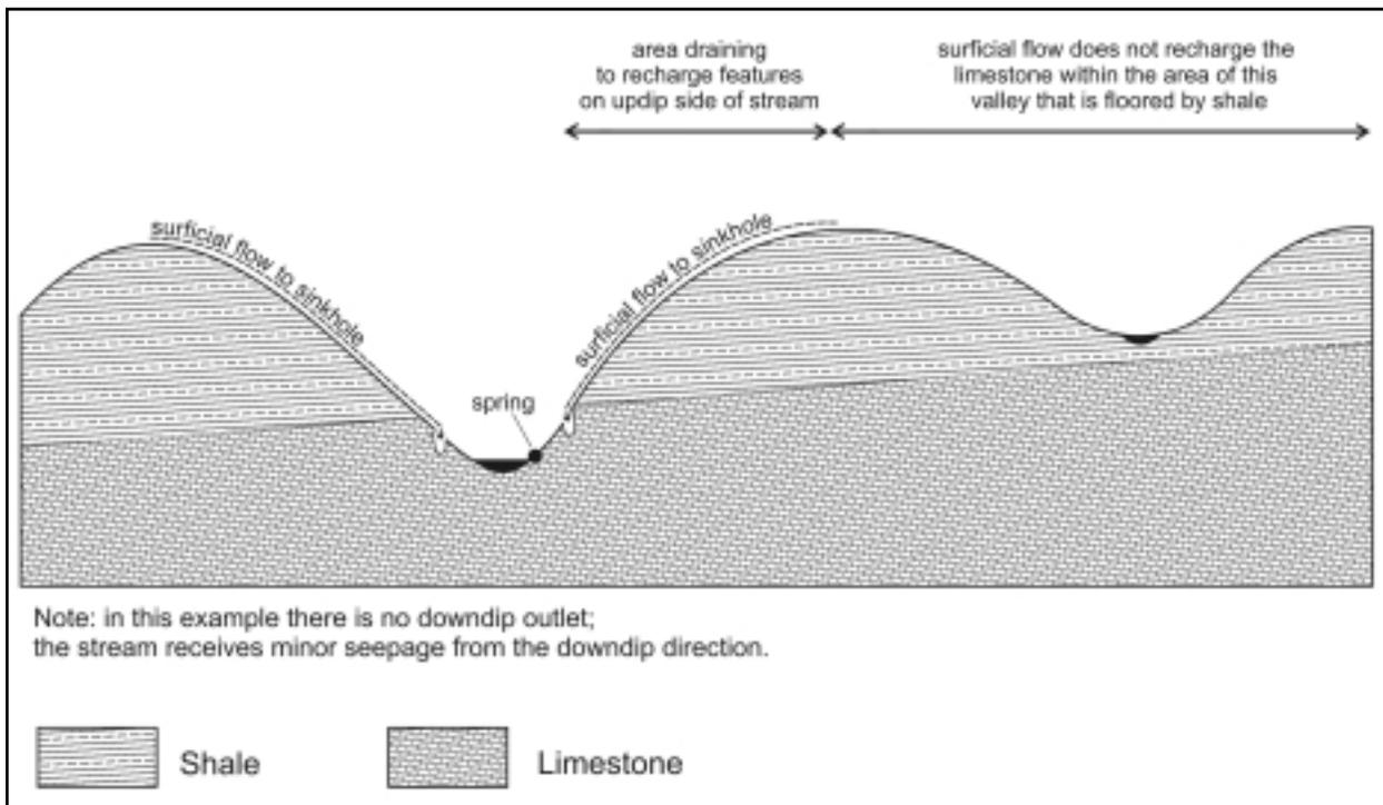
Figure 7. Cross section view of spring capture zone where the updip projection of the karst aquifer extends beyond the ridge, and the updip valley is separated from the underlying carbonate rock by an intervening thick shale.
