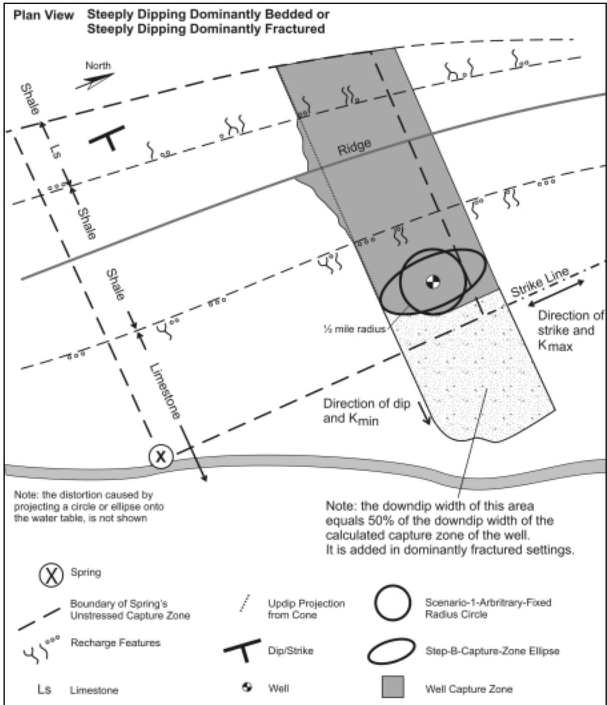
Figure 11. Capture zone of a well, located near the headward boundary of the spring's capture zone, in a steeply dipping aquifer, regardless of whether the aquifer is dominantly fractured or dominantly bedded.
