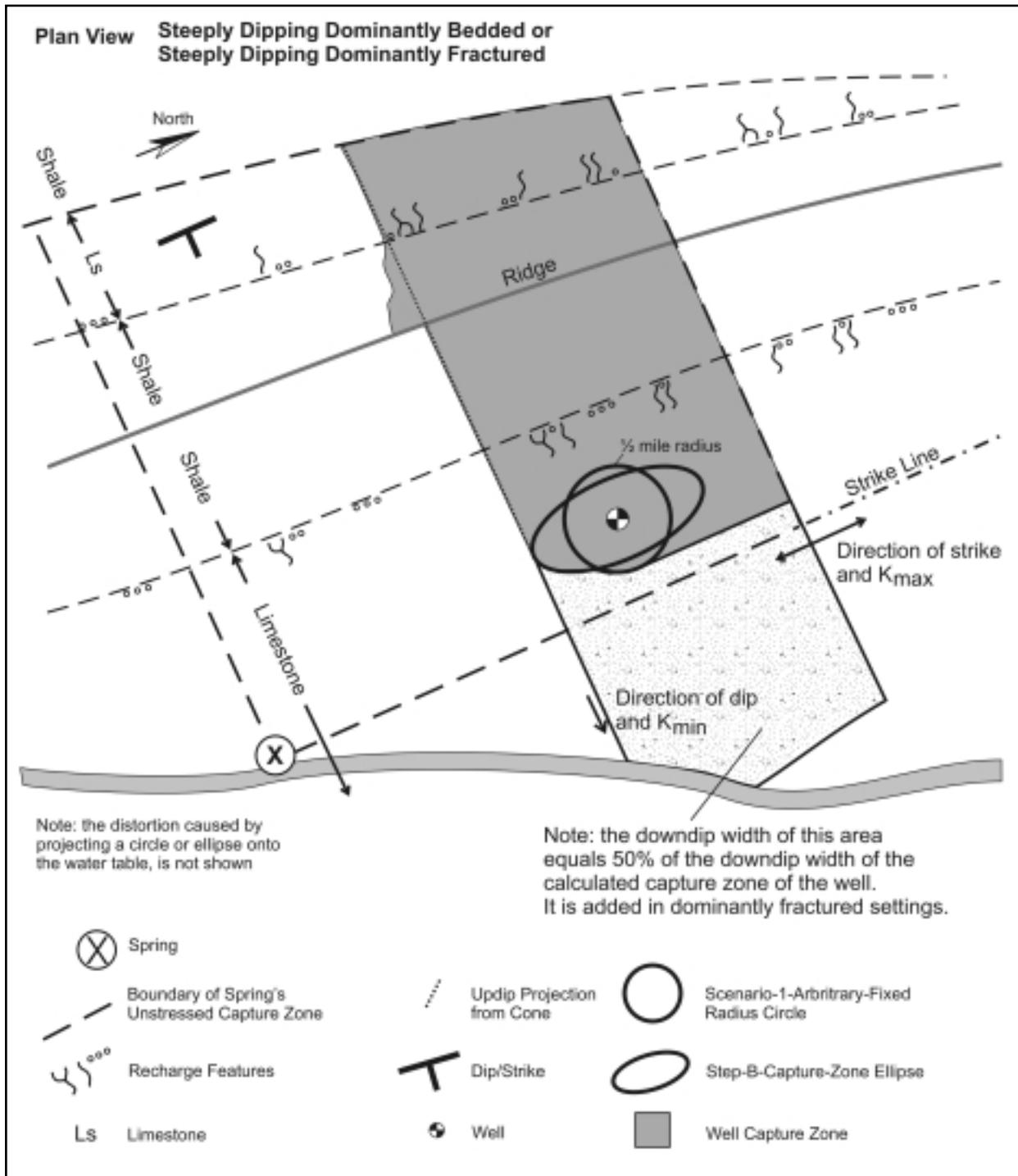
Figure 10. Capture zone of a well, located far enough from the headward boundary of the spring's capture zone that there is no interference, in a steeply dipping aquifer, regardless of whether the aquifer is dominantly fractured or dominantly bedded.
