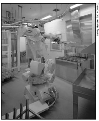
Figure 3. Robotics used in cage washing operation
