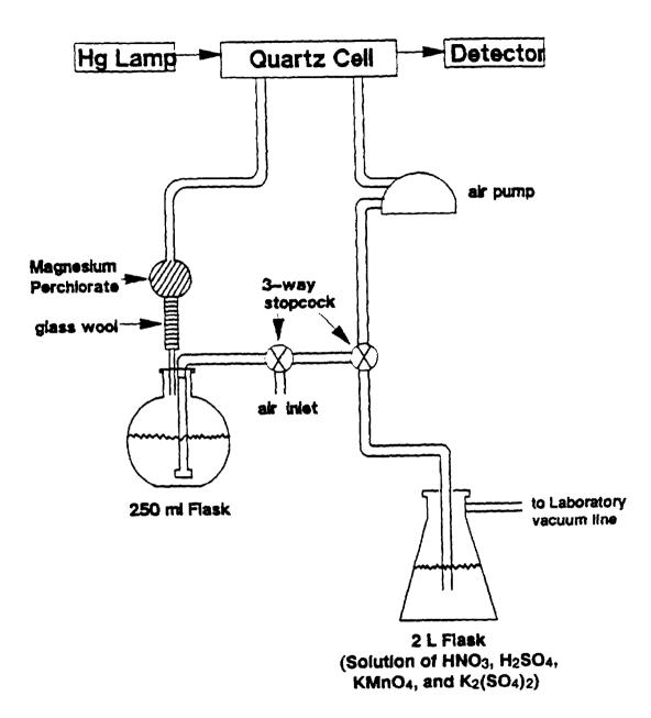
Figure 2-3. Schematic of laboratory analytical procedure for mercury.
