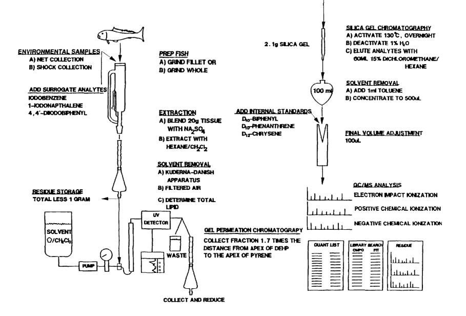
Figure 2-2. Schematic of laboratory analytical procedure for other xenobiotic chemicals.
