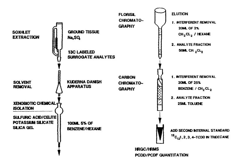
Figure 2-1. Schematic of laboratory procedures for dioxins and furans.
