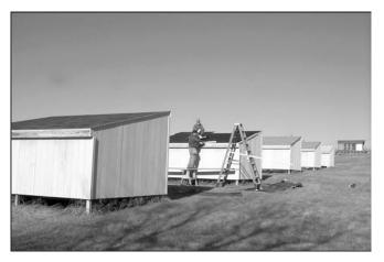
Figure 1—Exposure structures located at Forest Products Laboratory test site near Madison, Wisconsin. All five units were similar except for roofing materials and were instrumented for long-term temperature monitoring of roof assemblies. Shown, from the foreground, are black fiberglass shingles, western redcedar shingles (being installed), wood-thermoplastic composite shingles (two structures—closer with lath and further without lath), and white fiberglass shingles.
