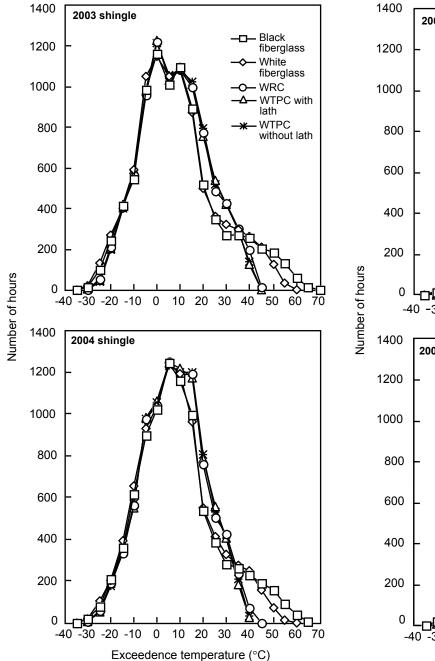
Figure 4—Cumulative temperature histories of WTPC (with and without lath), WRC, and fiberglass shingles exposed from January to December in 2003 and 2004 near Madison, Wisconsin.
