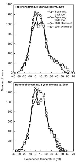
Figure 11—Cumulative temperature histories at top and bottom of sheathing in structures with black and white fiberglass shingles exposed from January to December 2004 compared to 8-year annualized data.
