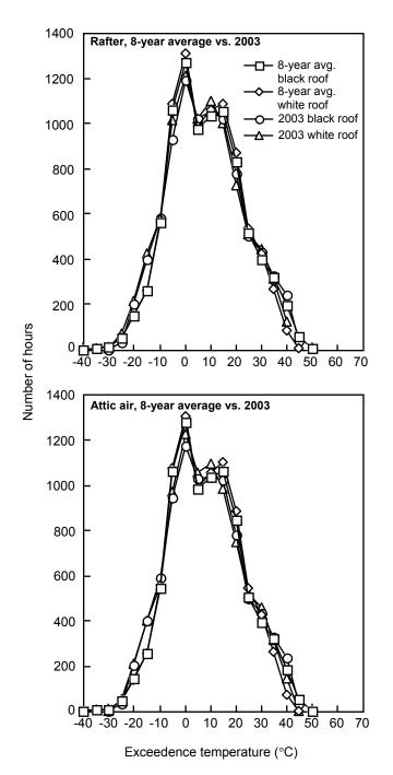
Figure 10—Cumulative temperature histories of rafters and attic air in structures with black and white fiberglass shingles exposed from January to December 2003 compared to 8-year annualized data.
