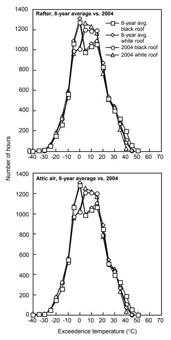
Figure 12—Cumulative temperature histories in rafters and attic air in structures with black and white fiberglass shingles exposed from January to December 2004 compared to 8-year annualized data.
