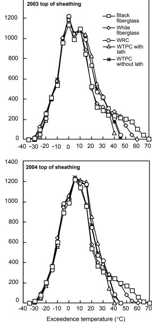
Figure 5—Cumulative temperature histories at top surface of roof sheathing under various types of shingles.
