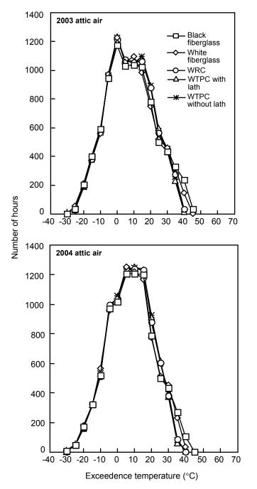
Figure 8—Cumulative temperature histories of attic air temperature in structures made with various types of shingles.
