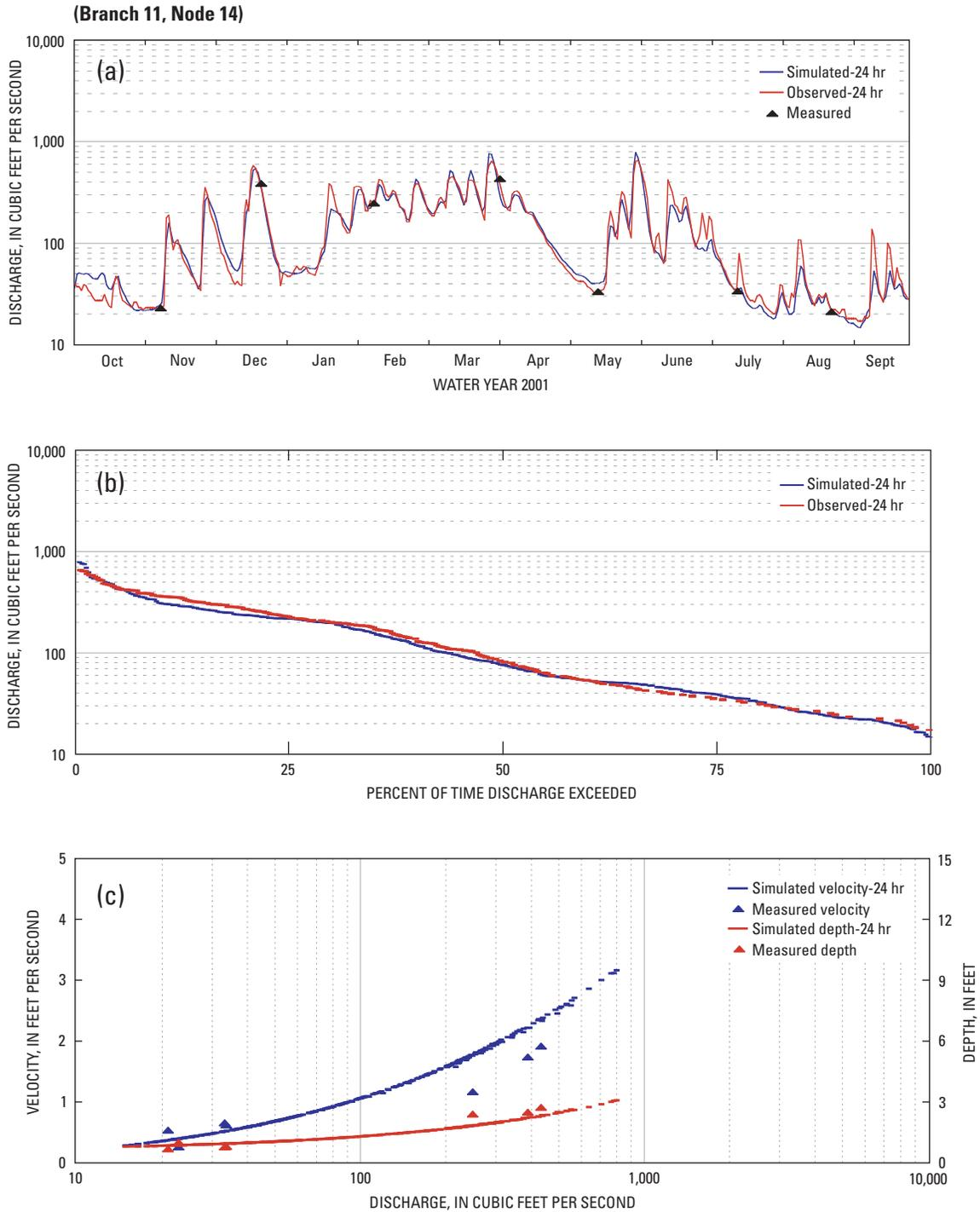
**Figure 9.** Calibrated (a) discharge, (b) flow duration, and (c) velocity and depth at gage 01379500, Passaic River near Chatham, New Jersey, water year 2001.
