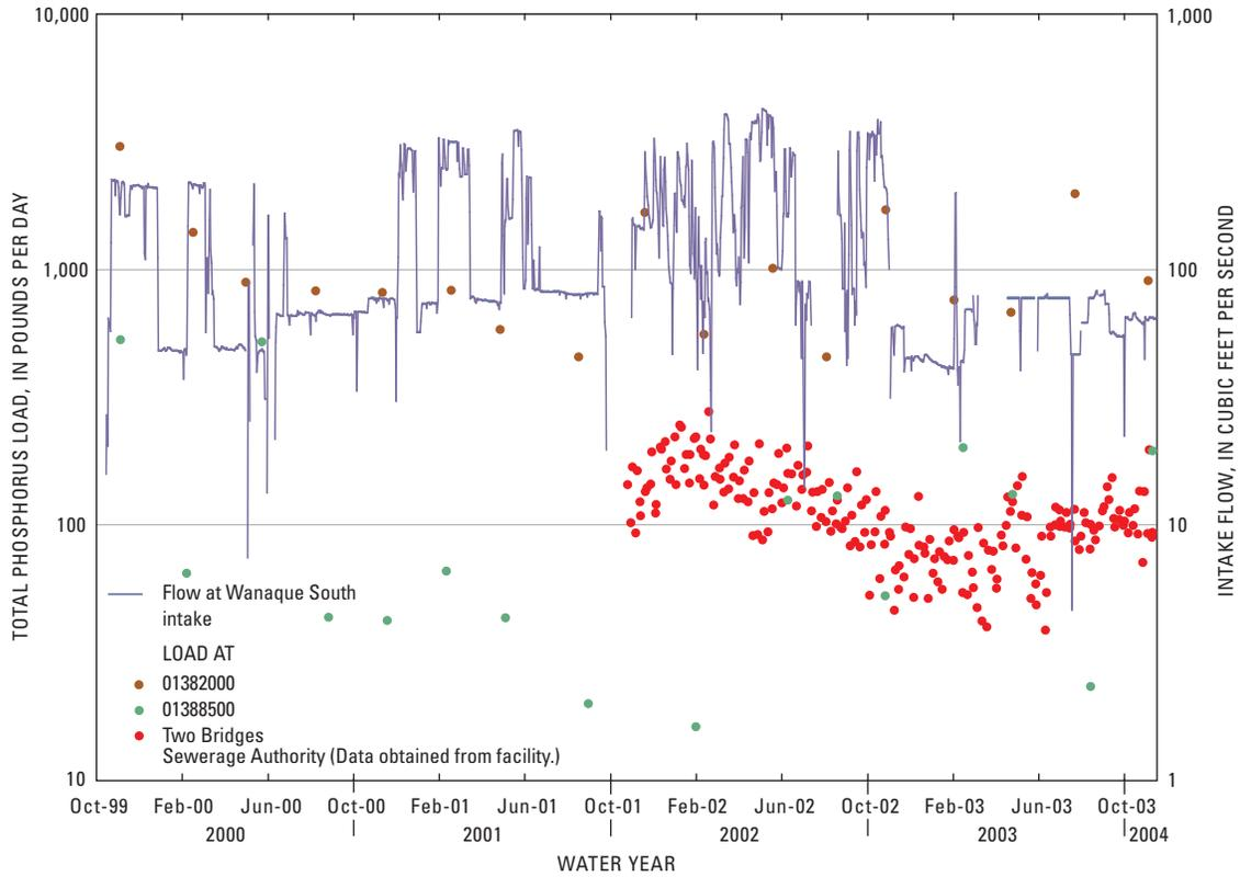
**Figure 32.** Intake flow and phosphorus loads in the vicinity of Two Bridges, New Jersey, 1999-2003. (Most locations shown in fig. 31)
