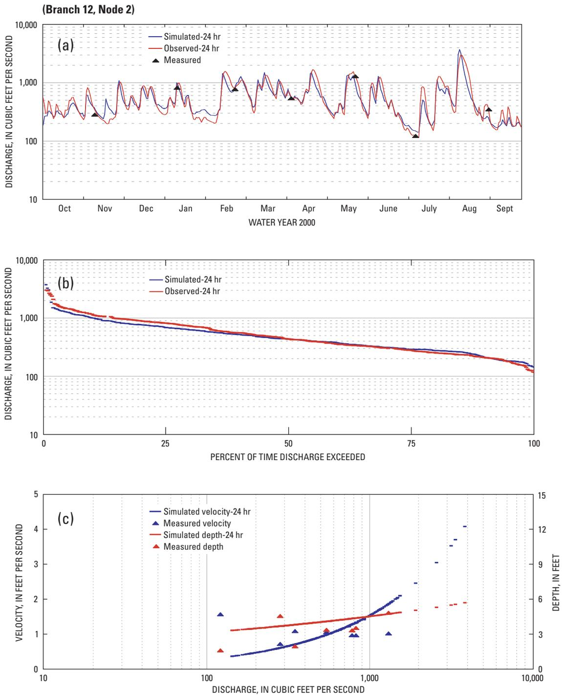
**Figure 16.** Validated (a) discharge, (b) flow duration, and (c) velocity and depth at gage 01381900, Passaic River at Pine Brook, New Jersey, water year 2000.
