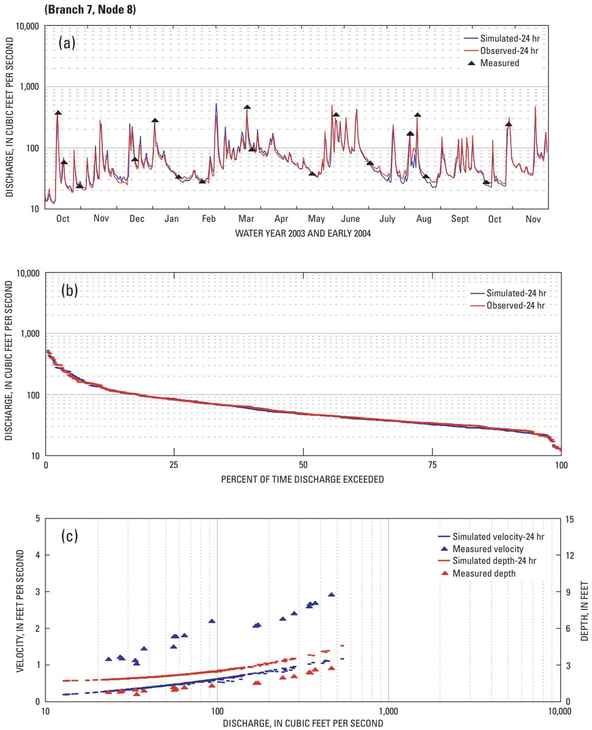
**Figure 26.** Validated (a) discharge, (b) flow duration, and (c) velocity and depth at gage 01381500, Whippany River at Morristown, New Jersey, water year 2003 and early 2004.
