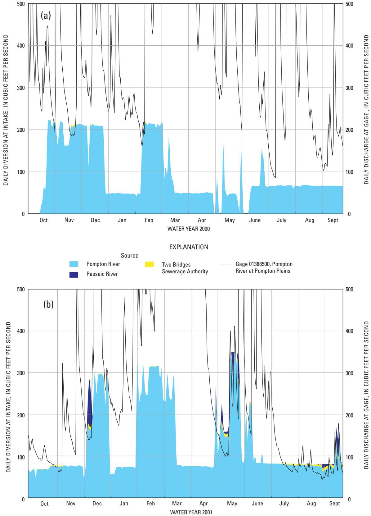
**Figure 34.** Simulated sources of water to Wanaque South intake, Two Bridges, New Jersey, for (a) water year 2000, (b) water year 2001, (c) water year 2002, and (d) water year 2003 and early 2004.
