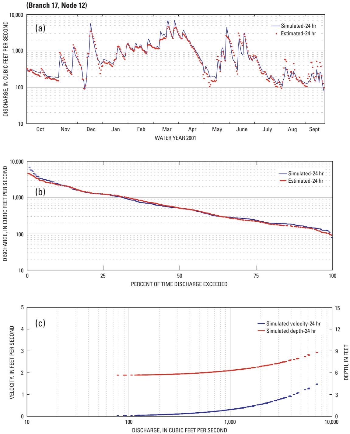
**Figure 12.** Calibrated (a) discharge, (b) flow duration, and (c) velocity and depth at station 01389890, Passaic River at Dundee Dam at Clifton, New Jersey, water year 2001.
