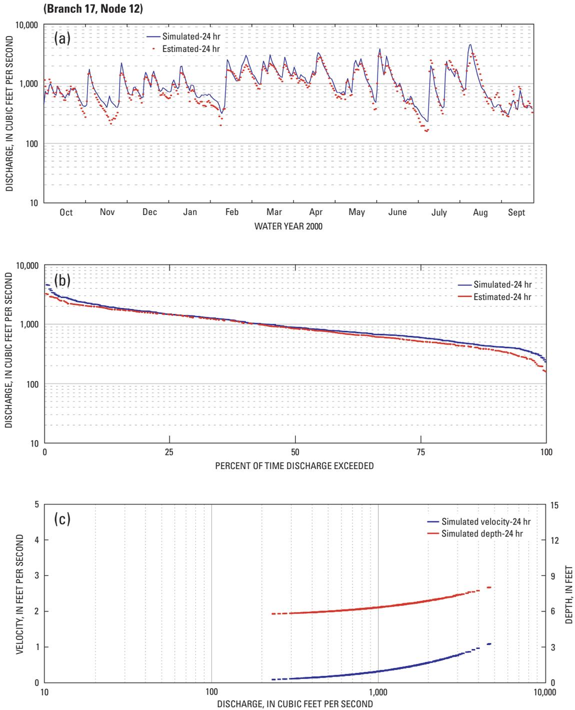
**Figure 18.** Validated (a) discharge, (b) flow duration, and (c) velocity and depth at station 01389890, Passaic River at Dundee Dam at Clifton, New Jersey, water year 2000.
