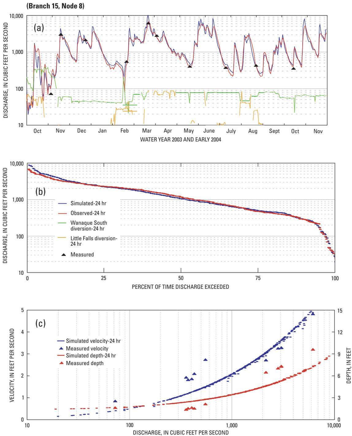
**Figure 29.** Validated (a) discharge, (b) flow duration, and (c) velocity and depth at gage 01389500, Passaic River at Little Falls, New Jersey, water year 2003 and early 2004.
