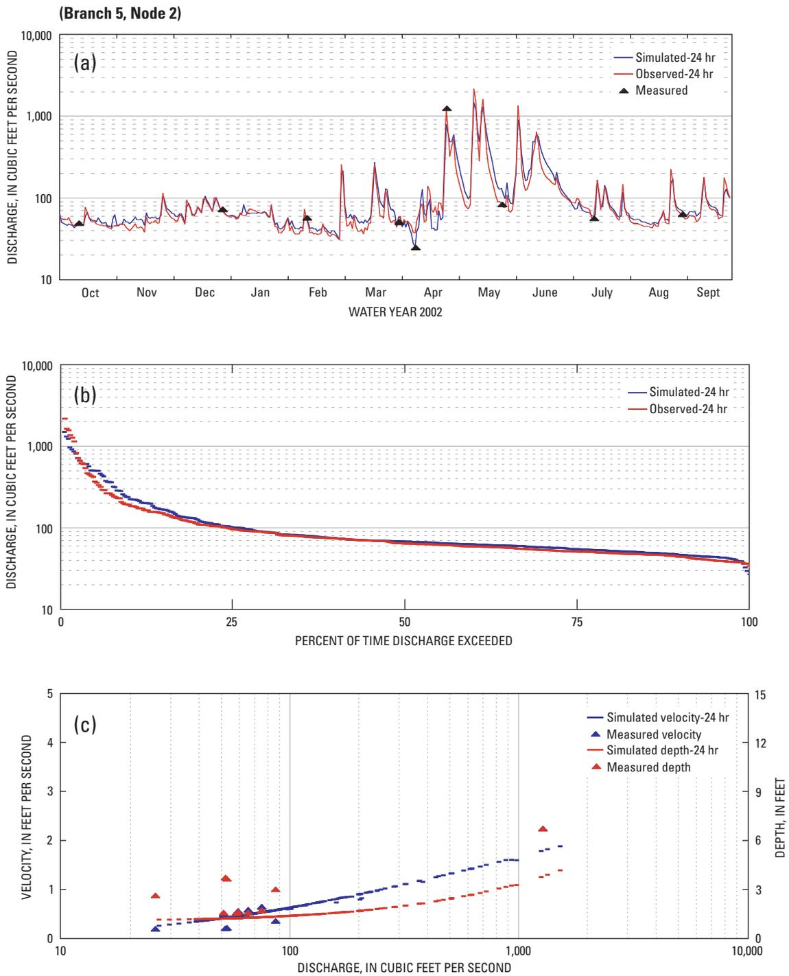
**Figure 19.** Validated (a) discharge, (b) flow duration, and (c) velocity and depth at gage 01388500, Pompton River at Pompton Plains, New Jersey, water year 2002.
