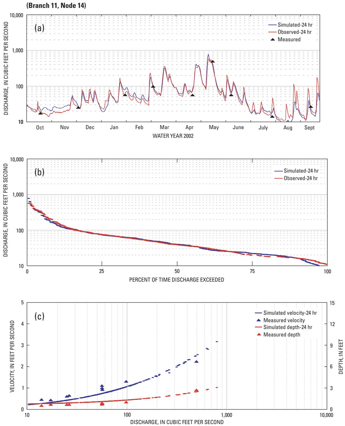
**Figure 21.** Validated (a) discharge, (b) flow duration, and (c) velocity and depth at gage 01379500, Passaic River near Chatham, New Jersey, water year 2002.
