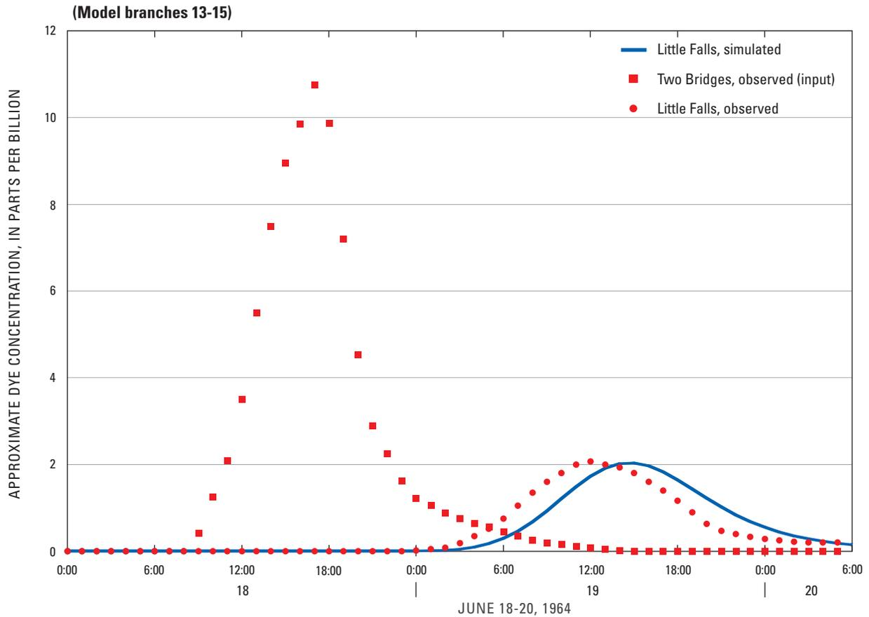
**Figure 35.** Calibrated dye transport between Two Bridges and Little Falls, New Jersey. (Observed data from Horwitz and Anderson, 1966.)
