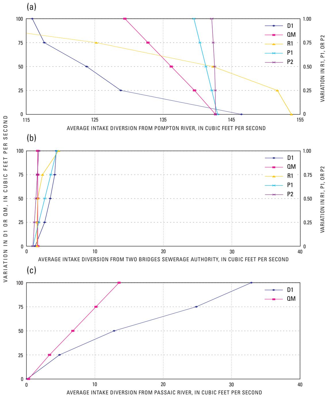
**Figure 33.** Results of sensitivity analysis on mixing algorithm parameters used in the flow model of the nontidal Passaic River, New Jersey, water year 2002. (Parameters D1, QM, R1, P1, and P2 identified on p. 56)
