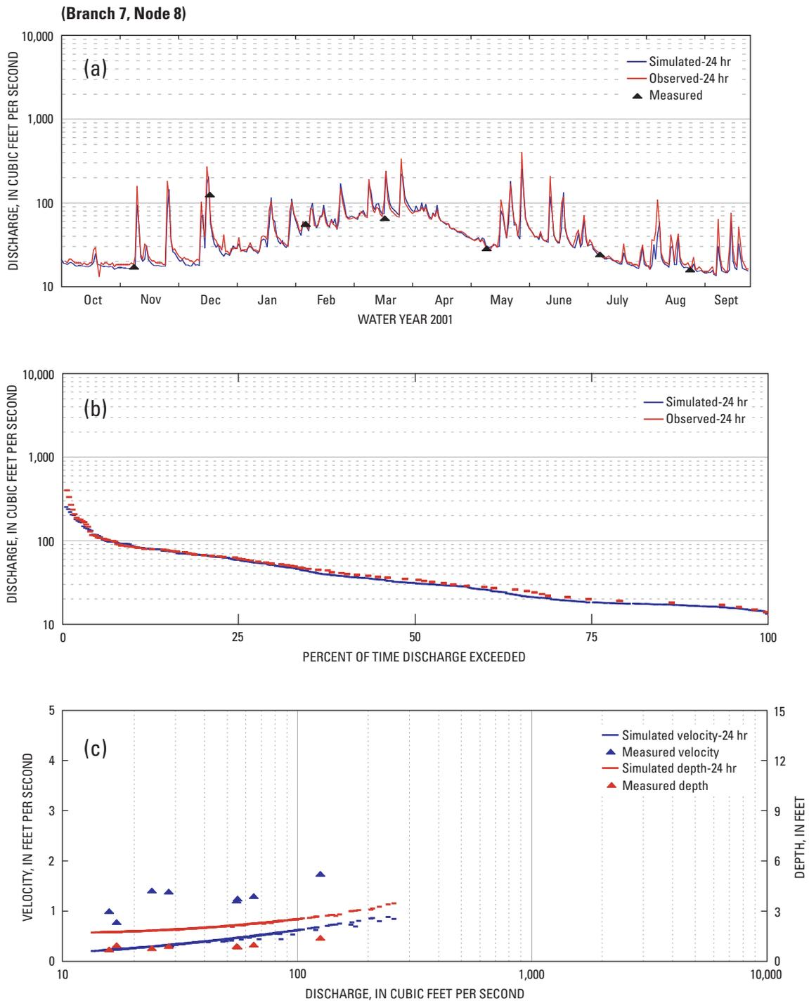
**Figure 8.** Calibrated (a) discharge, (b) flow duration, and (c) velocity and depth at gage 01381500, Whippany River at Morristown, New Jersey, water year 2001.
