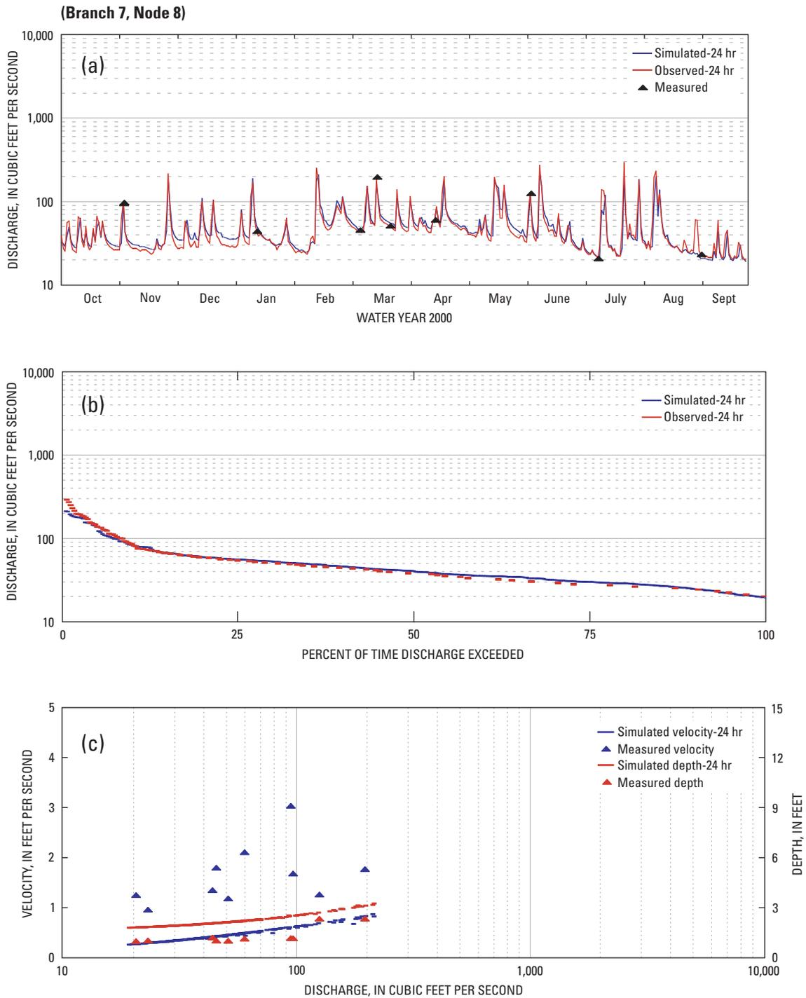
**Figure 14.** Validated (a) discharge, (b) flow duration, and (c) velocity and depth at gage 01381500, Whippany River at Morristown, New Jersey, water year 2000.
