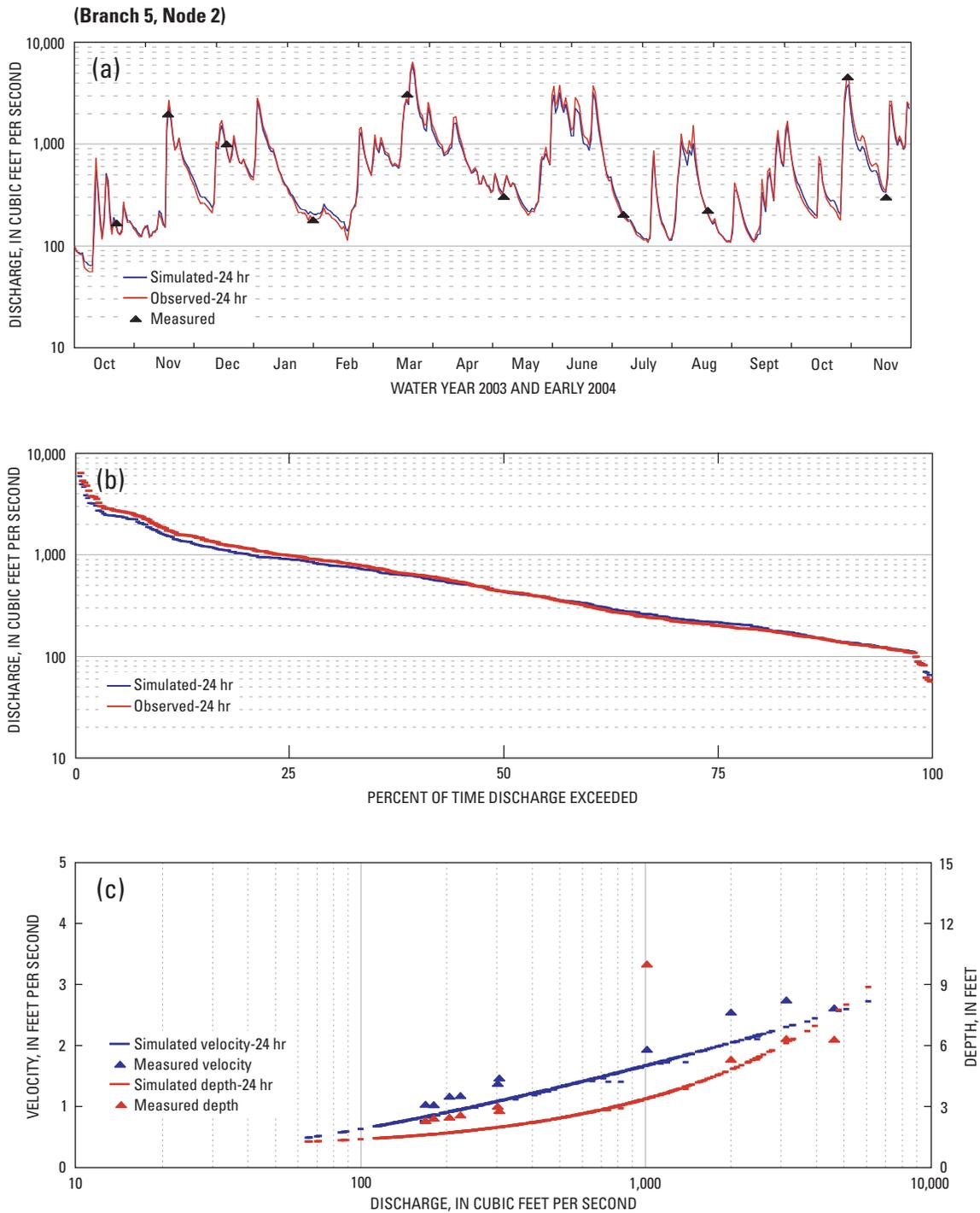
**Figure 25.** Validated (a) discharge, (b) flow duration, and (c) velocity and depth at gage 01388500, Pompton River at Pompton Plains, New Jersey, water year 2003 and early 2004.
