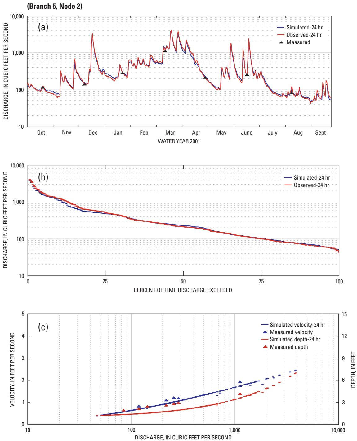
**Figure 7.** Calibrated (a) discharge, (b) flow duration, and (c) velocity and depth at gage 01388500, Pompton River at Pompton Plains, New Jersey, water year 2001.
