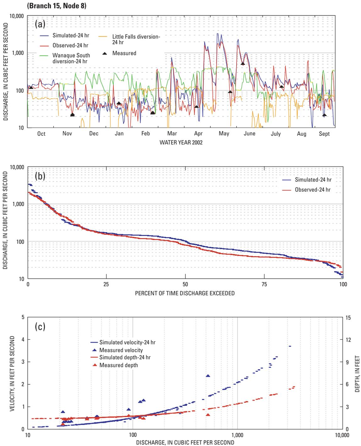
**Figure 23.** Validated (a) discharge, (b) flow duration, and (c) velocity and depth at gage 01389500, Passaic River at Little Falls, New Jersey, water year 2002.
