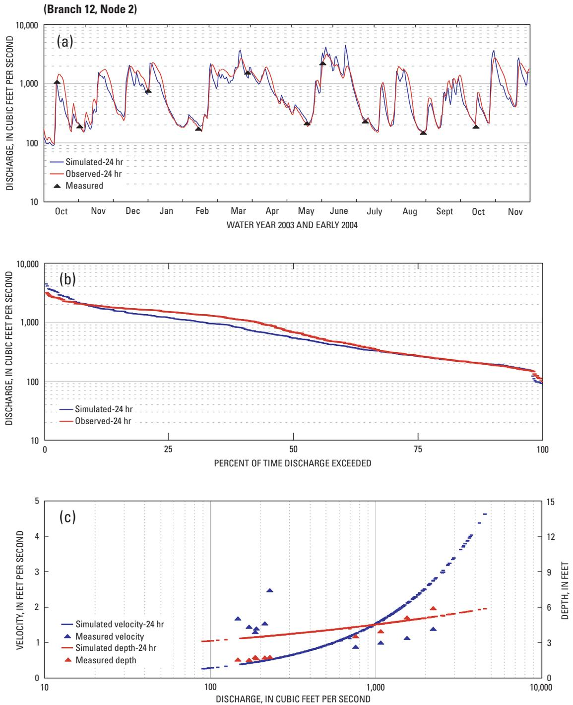
**Figure 28.** Validated (a) discharge, (b) flow duration, and (c) velocity and depth at gage 01381900, Passaic River at Pine Brook, New Jersey, water year 2003 and early 2004.
