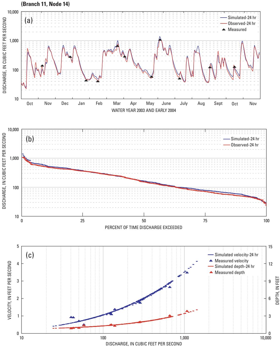
**Figure 27.** Validated (a) discharge, (b) flow duration, and (c) velocity and depth at gage 01379500, Passaic River near Chatham, New Jersey, water year 2003 and early 2004.
