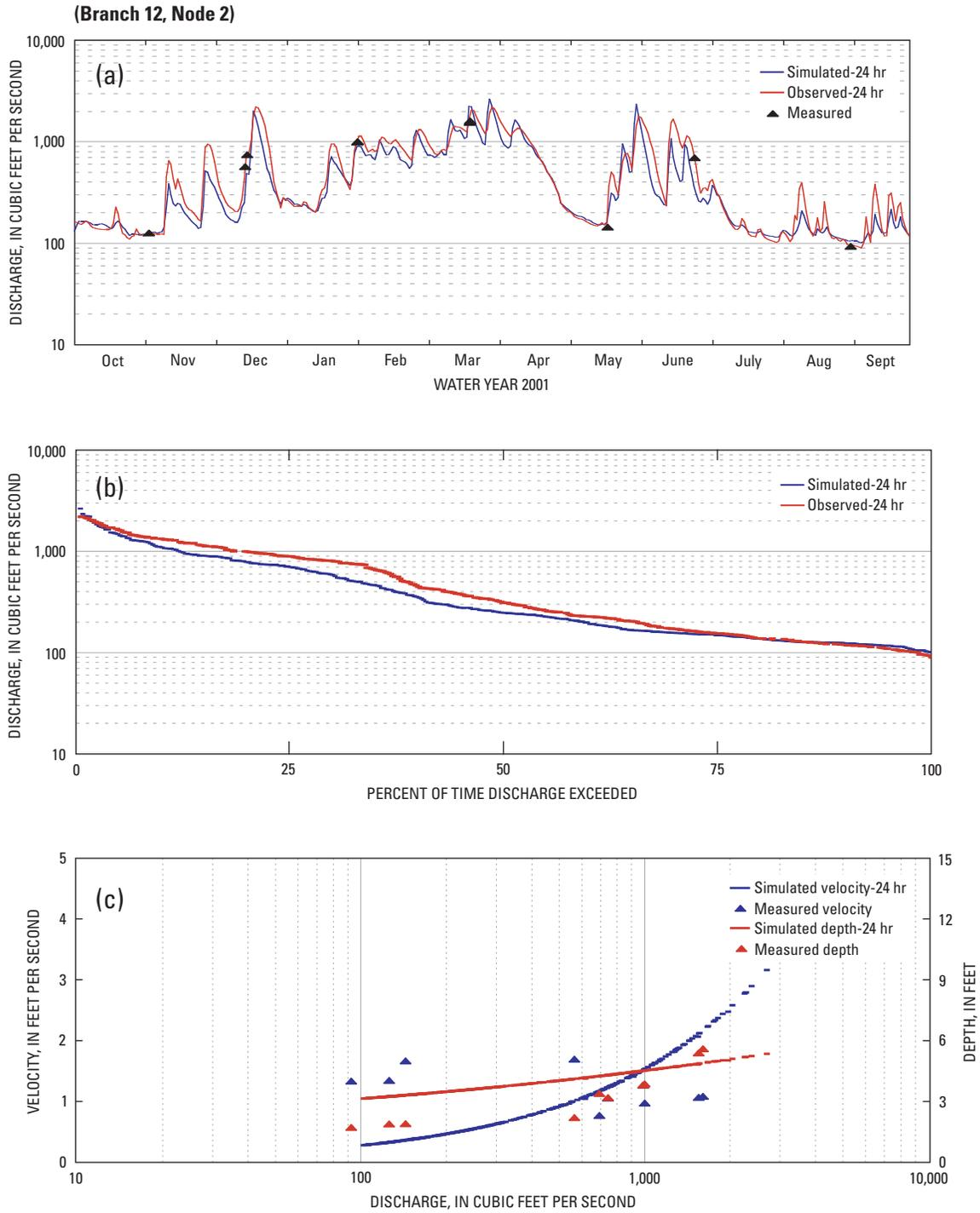
**Figure 10.** Calibrated (a) discharge, (b) flow duration, and (c) velocity and depth at gage 01381900, Passaic River at Pine Brook, New Jersey, water year 2001.
