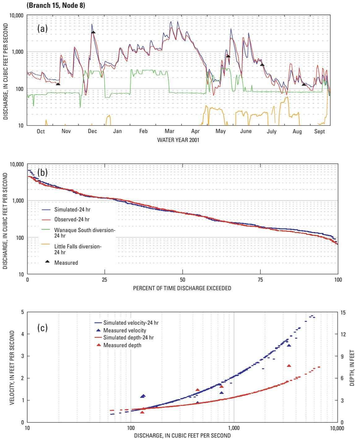
**Figure 11.** Calibrated (a) discharge, (b) flow duration, and (c) velocity and depth at gage 01389500, Passaic River at Little Falls, New Jersey, water year 2001.
