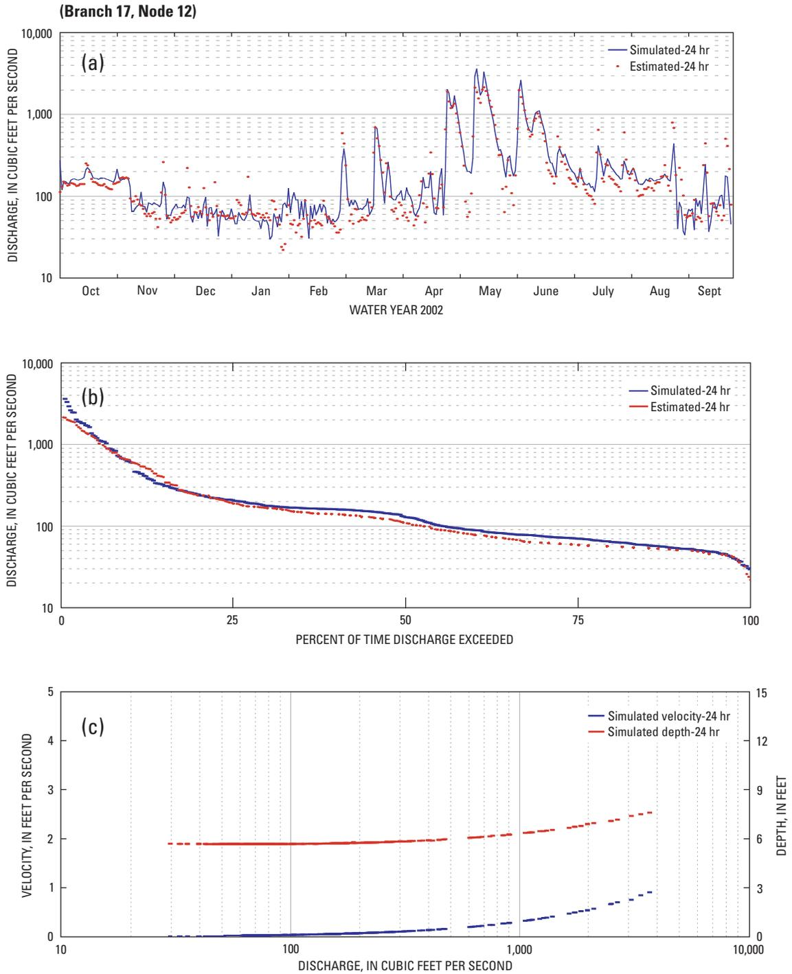
**Figure 24.** Validated (a) discharge, (b) flow duration, and (c) velocity and depth at station 01389890, Passaic River at Dundee Dam at Clifton, New Jersey, water year 2002.
