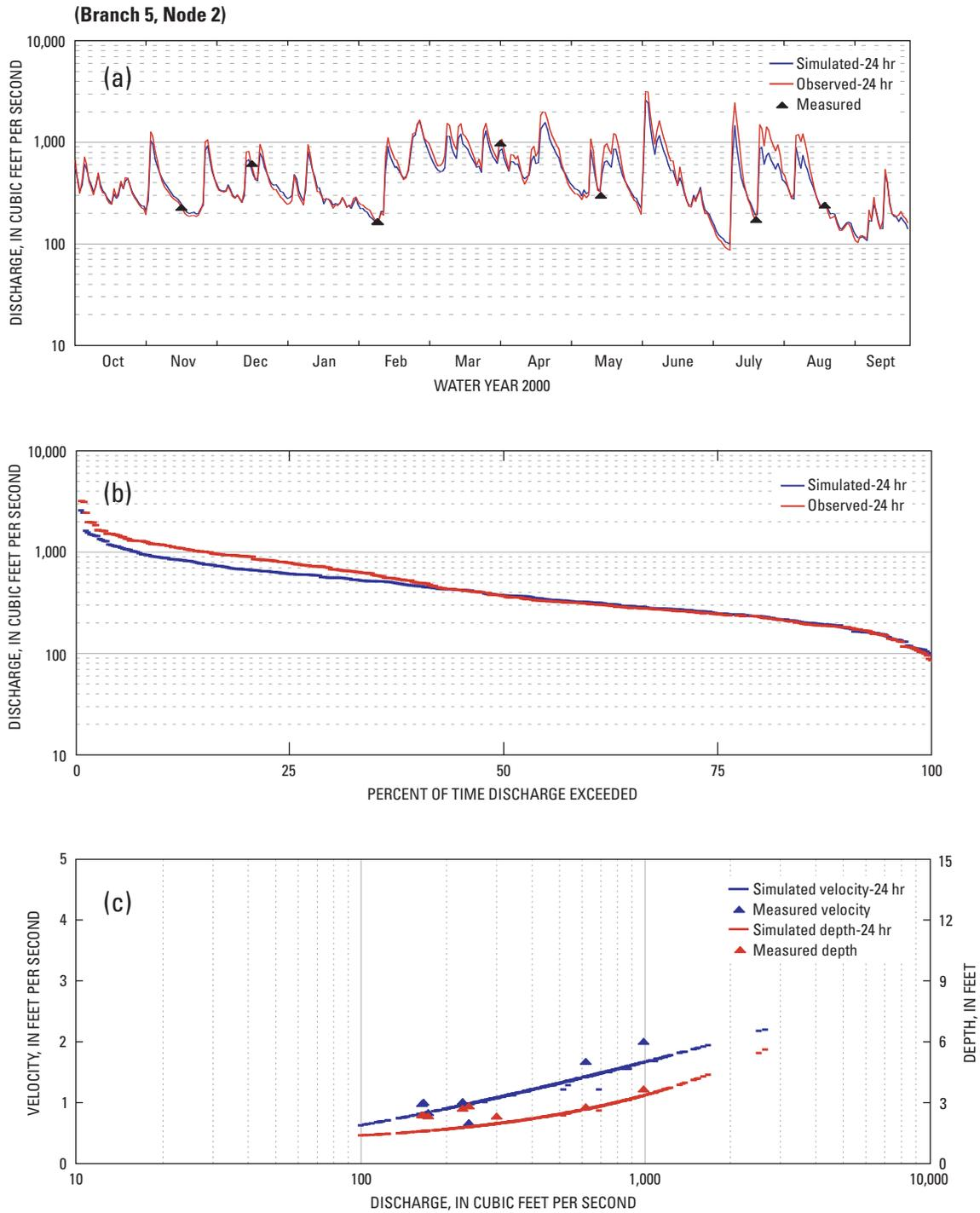
**Figure 13.** Validated (a) discharge, (b) flow duration, and (c) velocity and depth at gage 01388500, Pompton River at Pompton Plains, New Jersey, water year 2000.
