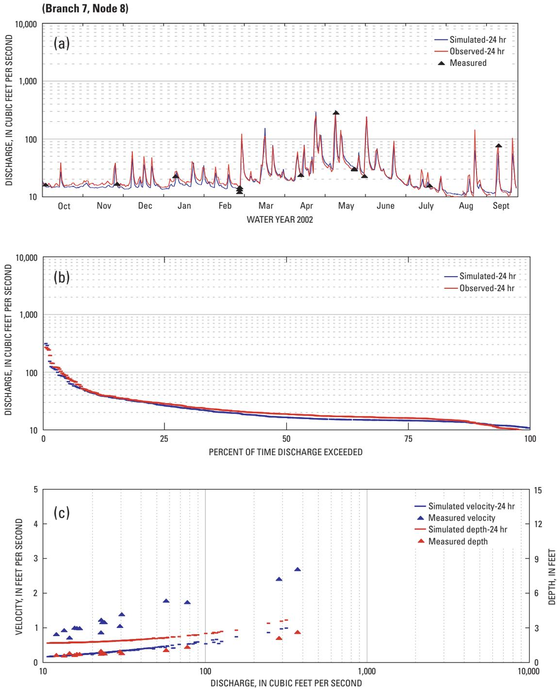
**Figure 20.** Validated (a) discharge, (b) flow duration, and (c) velocity and depth at gage 01381500, Whippany River at Morristown, New Jersey, water year 2002.
