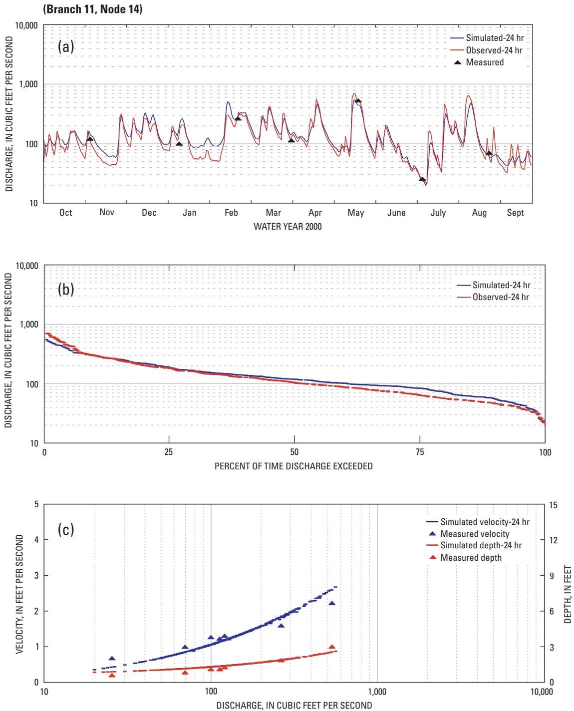
**Figure 15.** Validated (a) discharge, (b) flow duration, and (c) velocity and depth at gage 01379500, Passaic River near Chatham, New Jersey, water year 2000.
