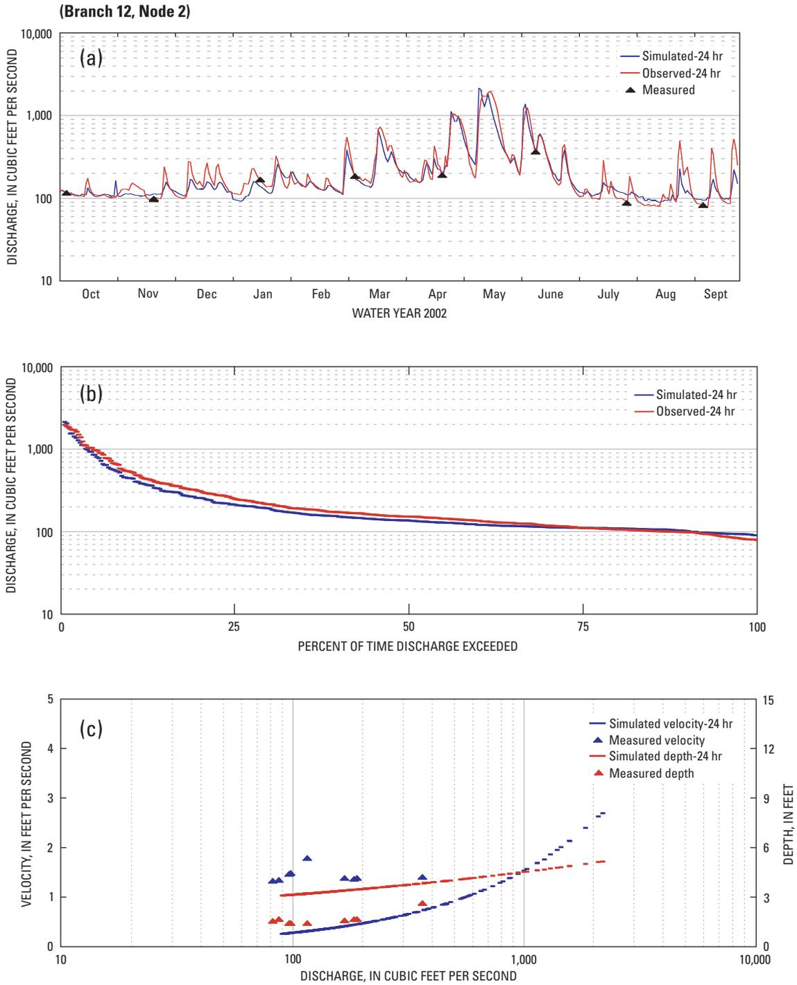
**Figure 22.** Validated (a) discharge, (b) flow duration, and (c) velocity and depth at gage 01381900, Passaic River at Pine Brook, New Jersey, water year 2002.
