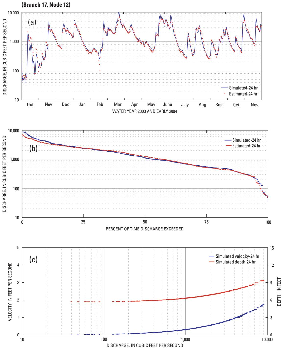
**Figure 30.** Validated (a) discharge, (b) flow duration, and (c) velocity and depth at station 01389890, Passaic River at Dundee Dam at Clifton, New Jersey, water year 2003 and early 2004.
