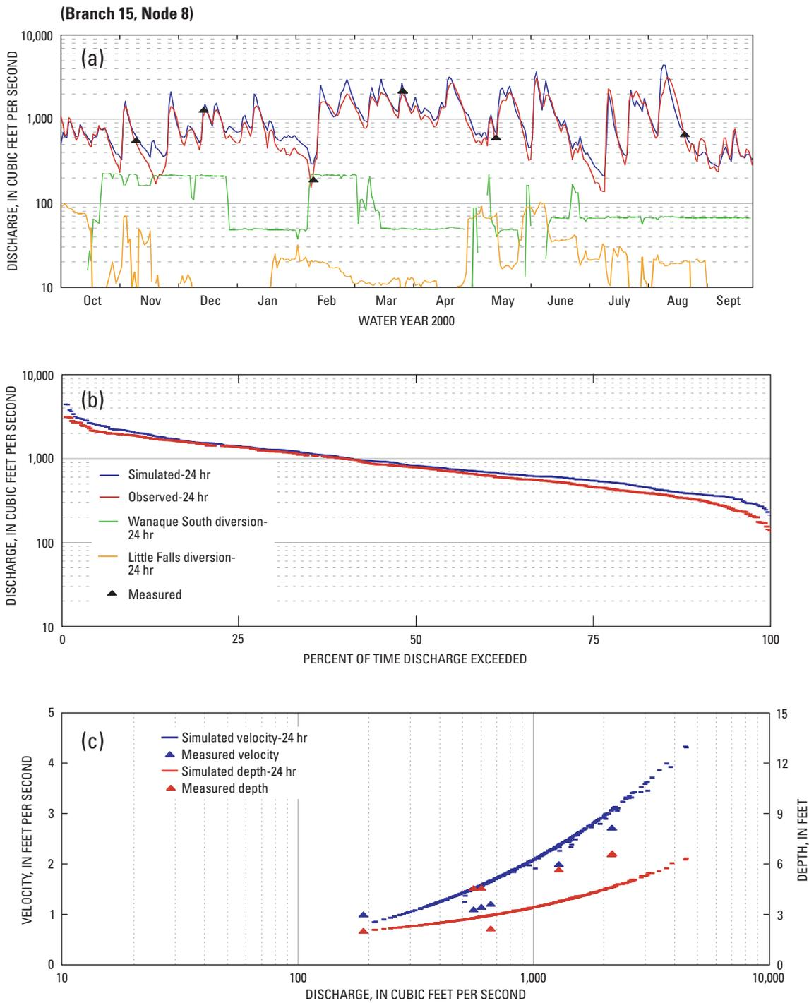
**Figure 17.** Validated (a) discharge, (b) flow duration, and (c) velocity and depth at gage 01389500, Passaic River at Little Falls, New Jersey, water year 2000.
