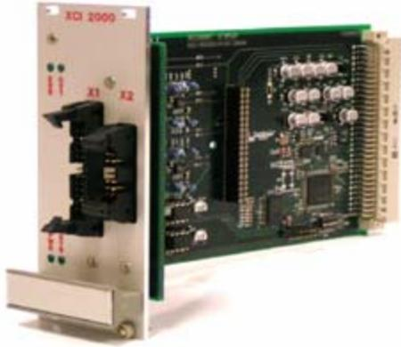
Figure 20. XCI 2000 four-phase converter control card
