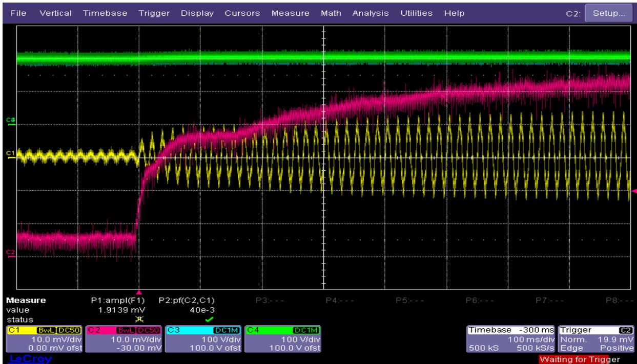
Figure 48. Transient from 1 A to 10 A of DC-link current at  $\langle V_{dc} \rangle = 328$  V, 1464 rpm
