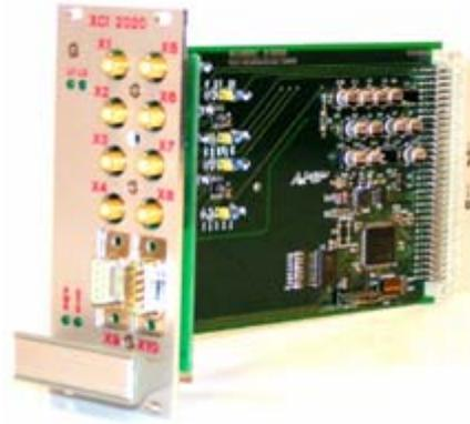
Figure 21. XCI 2020 universal input/output card
