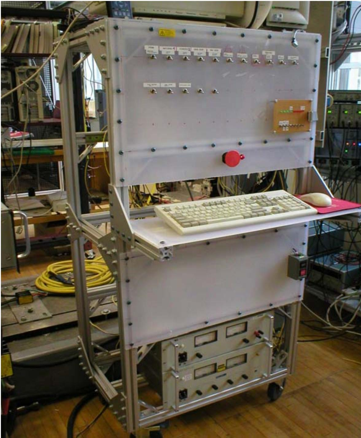
**Figure 25. Detail of the control panel for the entire prototype. The PC is used to program and set the references to the DSP controller, as well as to collect the measurement from the oscilloscopes**
