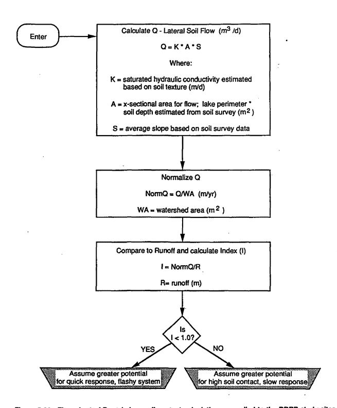
Figure 5-29. Flow chart of Darcy's Law soil contact calculation as applied to the DDRP study sites.
