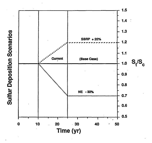
Figure 5-27. Sulfur deposition scenarios for the NE and SBRP for Level II and III Analyses. Ration of total sulfur deposition at time t ( $S_t$ ) to current total sulfur deposition ( $S_c$ ).
