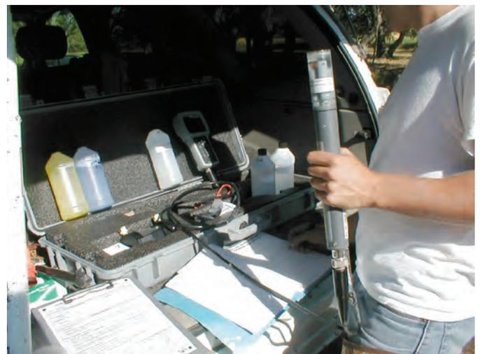
**Figure 13.** Crew members calibrated water-quality instruments prior to collecting field measurements.
