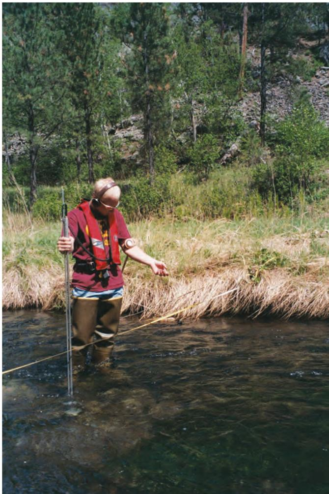
**Figure 8.** A field crew member making a stream discharge measurement at the “X-site.”
