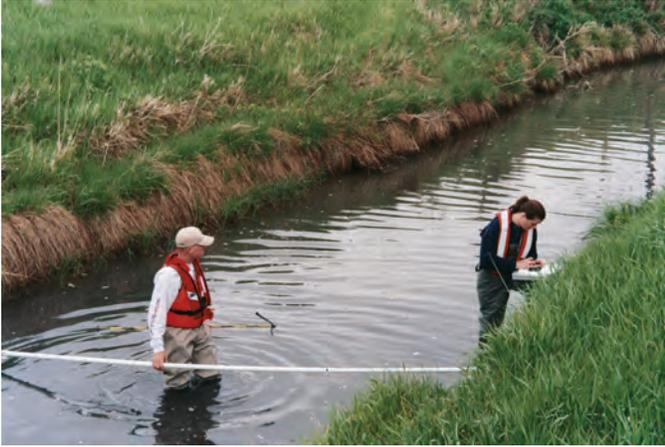
**Figure 7.** Field crew members measured the wetted stream width to determine channel dimensions throughout the designated stream assessment reach.
