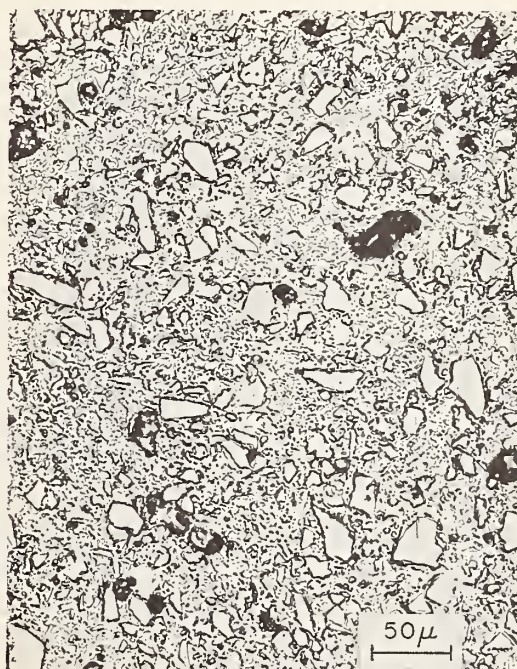
FIGURE 2. Electrical insulator porcelain with low quartz grain dissolution (etched 10 sec, 0 °C, 40% HF, collodion replica).
