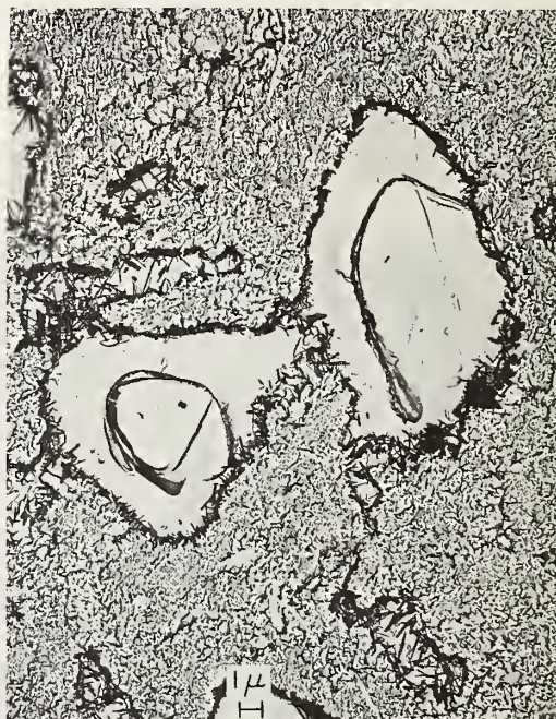
FIGURE 16. Partly dissolved quartz grains with microstress cracks (fracture surface, silica replica).
