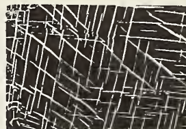
FIGURE 8. Widmanstätten structures. Example: \text{UC}_2 (bright) in UC (X281). [Chang, R., and C. G. Rhodes, "High-Pressure Hot-Pressing of Uranium Carbide Powders and Mechanism of Sintering of Refractory Bodies," J. Am. Ceram. Soc. 45 , 379 (1962)].
