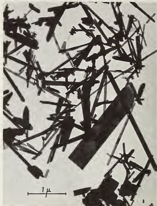
FIGURE 8. Isolated and dispersed mullite phase of an insulator porcelain.
