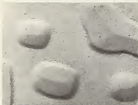
FIGURE 9. Domains. Example: \text{BaTiO}_3 aligned with the c-axes perpendicular to the figure (X5625). Etched by \text{H}_3\text{PO}_4 . The positive ends etched more rapidly than the negative ends. [Belitz, R. K., "Differential Etching of \text{BaTiO}_3 by \text{H}_3\text{PO}_4 ," J. Am. Ceram. Soc. 45 , 617 (1962)].
