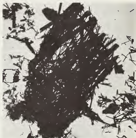
FIGURE 9. Stereoscopic views of a part (the large aggregate) of the mullite phase from a feldspar relict region showing the magnitude and relative position of the mullite crystals. To the left some smaller, more compact aggregates from clay relicts can be seen.
