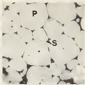
FIGURE 27. Grain separation. Example: periclase ( \text{MgO} ) and an \text{MgO} -saturated calcium silicate liquid (approx. X140). Although less than 10 percent liquid is present, it allows only a negligible quantity of solid-to-solid contact (Cf. fig. 28, fig. 2c, and fig. 11b.) [21] P - periclase; S - silicate liquid.
