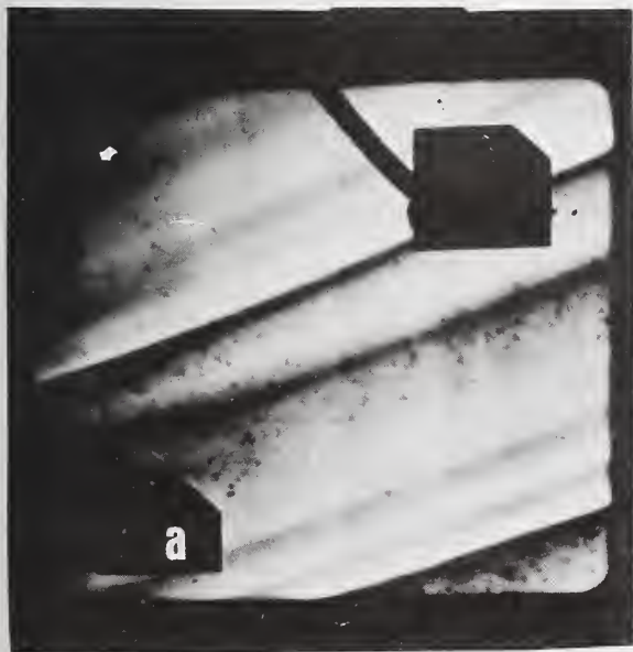
Figure 20. Electron beam induced current response (a) and unmodulated 0.633\text{-}\mu\text{m} laser beam induced current response (b) of a 0.76\text{-mm} square, unbiased, silicon p - n junction diode. (Scanning electron micrograph, EBIC mode, by K. O. Leedy.)
