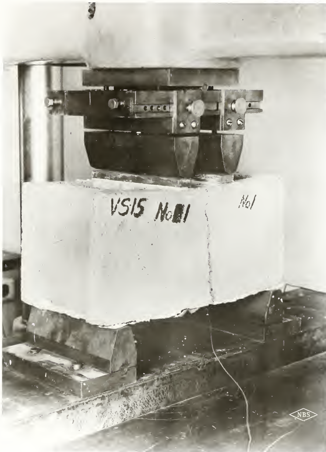
Figure 3- Flexure load specimen, after test.
