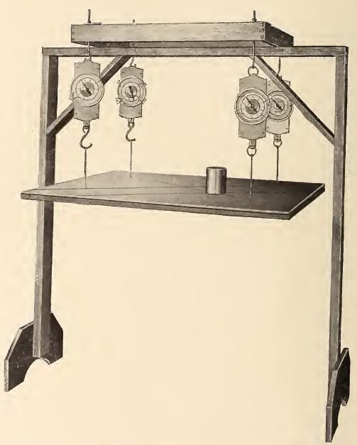
Fig. 5.—Apparatus to show the distribution of load among the four corner supports of a rigid platform.
