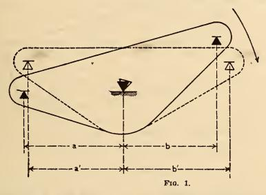
is not constant the scale can be made to give correct weights for some particular load but will not be right for other loads. This defect, in general, will arise from sources brought about by deflection of the supports and flexure of the parts. These sources will be divided into three kinds:
