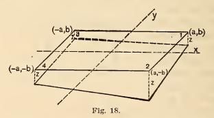
platform. In other words, we must locate the center of the four corner forces, or must find the point at which the resultant force is located. This point corresponds to the position of the load.
