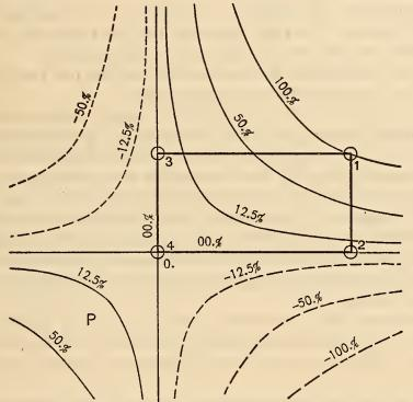
Fig. 9.-Lines of constant weight for corner 1 for a platform of the flexible type.
