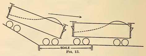
truck to the other. To illustrate the point, an extreme in the other direction may be considered in which the center of gravity C is so low as to be on the line F R. In this case there would be no shift of load from one truck to the next with a change in grade.
