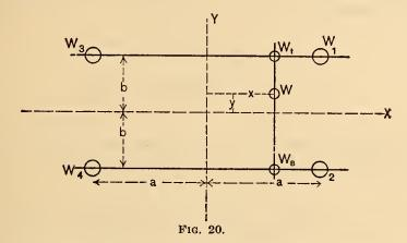
Examining the change in the portion of the weights carried by corner 1 as we move the load from corner 4 along the diagonal in the direction of corner 1 we have for points along the diagonal
