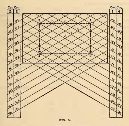
A complete chart from which can be found the portion of the load carried at each support for any given position of the load is given in figure 4.
