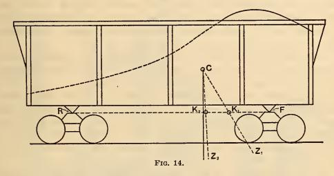
weight obtained by adding the result of the two truck weighings would be in error by the amount that the second truck had gained or lost while being placed in position. In other words the error is not due to any particular distribution of the load between the trucks but to changes in this distribution that occur between the separate weighings.
