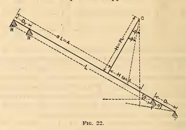
A =Distance of the c. g. measured along the car from the second truck.
