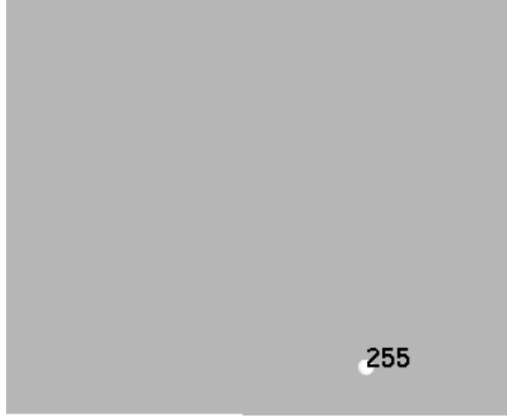
Figure 3.1: A test verifying that Smokeview can correctly transform the physical (x,y,z) location of the smoke_sensor object to its equivalent screen coordinates where the underlying smoke obscuration level is retrieved. A small white (255,255,255) smoke_sensor appears in front of a grey (128,128,128) obstacle. The value displayed should be 255, the value recorded by Smokeview. If the physical to screen transformation is performed incorrectly a value of 128 will be displayed (since it will pick up a color elsewhere).
