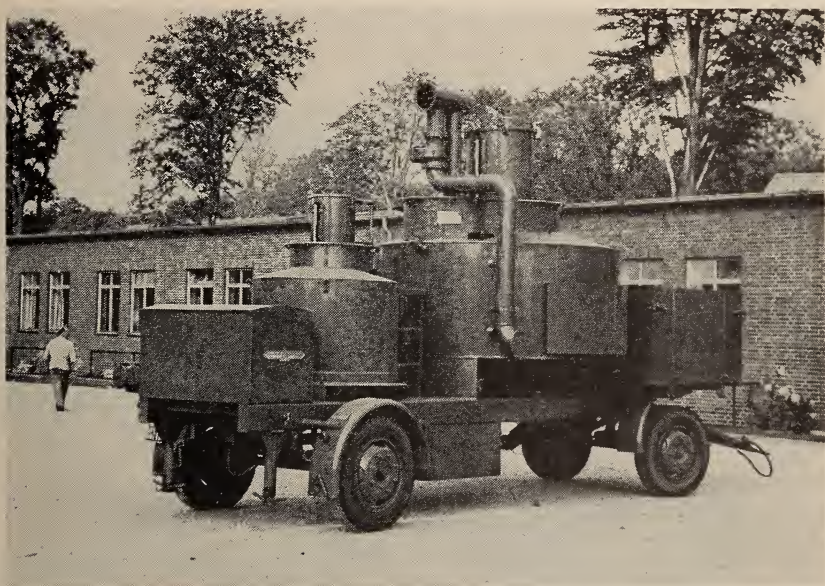
Volumetric test vehicle with two test measures of high accuracy for 1000 liters and 5000 liters built by the Schwelmer Eisenwerk for PTB. Similar test measures are used by the State Metrology Boards to test tanks, pumps, and volumetric meters.
