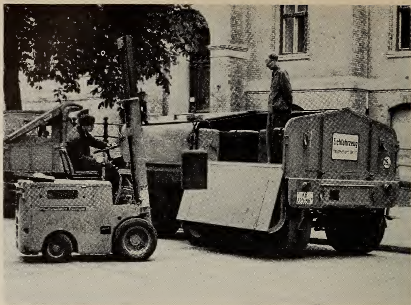
Test vehicle of the Metrology Board of Berlin used as a standard load for testing road and vehicle scales.
