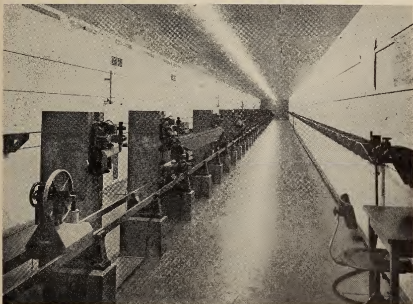
60 meter comparator room in which are tested measuring tapes and line standards using optical and photoelectrical methods. Smaller comparators of this kind are installed in the State Metrology Boards and in some Metrology Offices.
