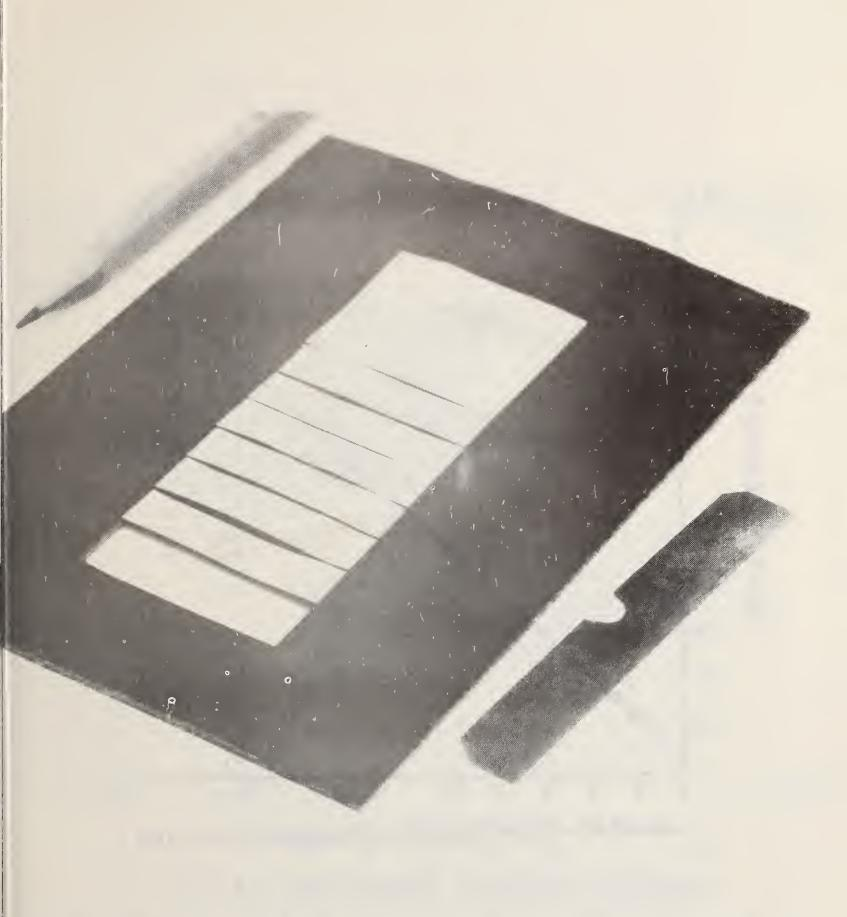
Figure 4: Two exposure aids used in the production of edge-artifacts. On the right is the tantalum strip used to produce the sharp edge-discontinuity. The right edge of the strip has received a metallographic polish. On the left is a typical 7-step tablet of aluminum foil layers. In use, the layers are tightly compacted; here they have been slightly separated to exhibit the format. Typical transmittance factors for such a tablet with x-rays are shown in Tables I and IV.
