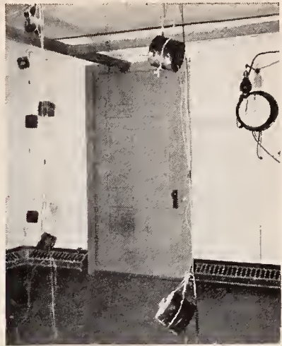
Left: the thermal conductivity of cement is measured in a Bureau laboratory. Right: baseboard heating elements for buildings were studied (p. 69) in the Bureau's test bungalow. Note the thermocouples suspended from the ceiling for measurement of temperatures at various heights.
