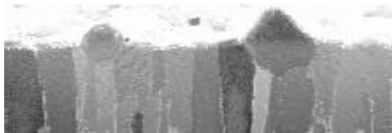
Figure 27. Scanning electron micrograph view of a cross section of a tin electrodeposit containing hillocks. There is evidence of grain boundary motion in the deposit under each hillock.
