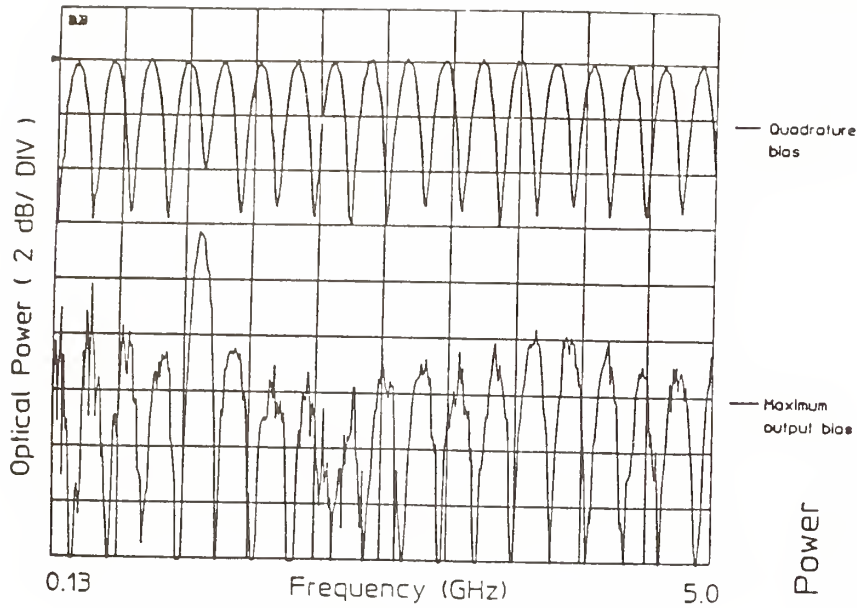
Fig. 2: Frequency response of the AM and PM modulation of the LiNbO 3 Mach-Zehnder interferometer biased at quadrature (upper curve) and maximum output (lower curve).
