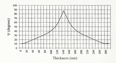
Figure 3:  $\psi$  Values at 70° Angle of Incidence First Thickness Cycle  $\lambda = 632.8, n_f = 1.460$
