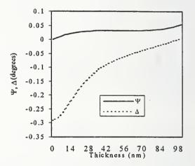
Figure 1. Change in  $\Delta$  and  $\psi$  with a 0.05° change from 70° in the angle of incidence for different  $SiO_2$  film thicknesses.
