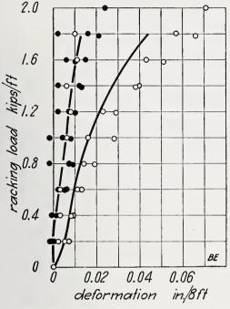
FIGURE 16.—Racking load on wall BE.
