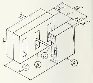
FIGURE 1.—"Dun-Ti-Stone" concrete unit. A, facing slab; B, backing slab; C, recess; D, tie bar.
