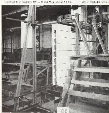
FIGURE 15.-Wall specimen BE-R1 under racking load.
