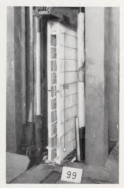
FIGURE 3.—Wall specimen BE-C1 under compressive load.
