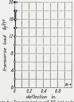
FIGURE 8.—Transverse load on wall BE, load applied to outside face.
