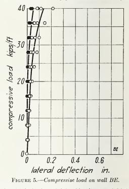
Load-lateral deflection (open circles) and load-lateral set (solid circles) results for specimens BE-C1, C2, and C3. The load was applied 2.81 in. from the inside face. The loads are in kips per foot of actual width of specimen. The deflections and sets are for a gage length of 6 ft 5 in., the gage length of the deflectometers.
