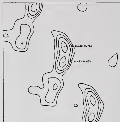
Figure 8. Difference-Fourier map for kaolinite-hydrazine showing the N_2H_4 molecule represented by the two largest peaks at (0.38, 0.39, 0.723) and (0.467, 0.483, 0.655) in the interlayer space. Contours are drawn at 0.15, 0.30, 0.45, and 0.65 electrons. The c axis is approximately vertical.
