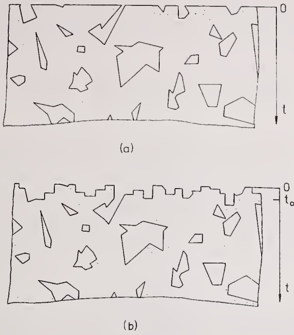
Figure 3: Simulation of surfaces of porous materials by intersecting a Boolean model. (a) Smooth surface produced by a smooth planar section through the infinitely extended model. (b) Rough surface generated by a fuzzy planar section of the Boolean model.
