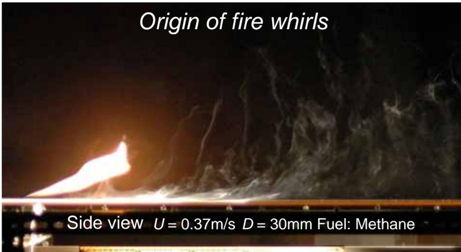
Side view  $U = 0.37\text{m/s}$   $D = 30\text{mm}$  Fuel: Methane
