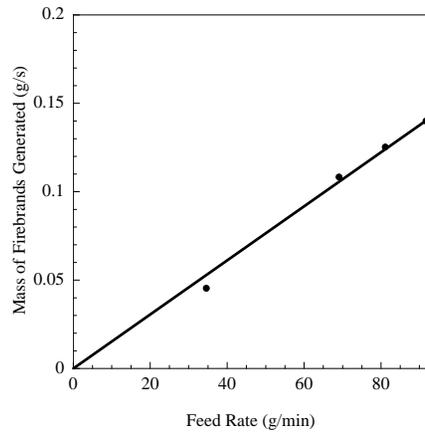
Generation rate (g/s) was linear and increased with an increase in wood feed rate
