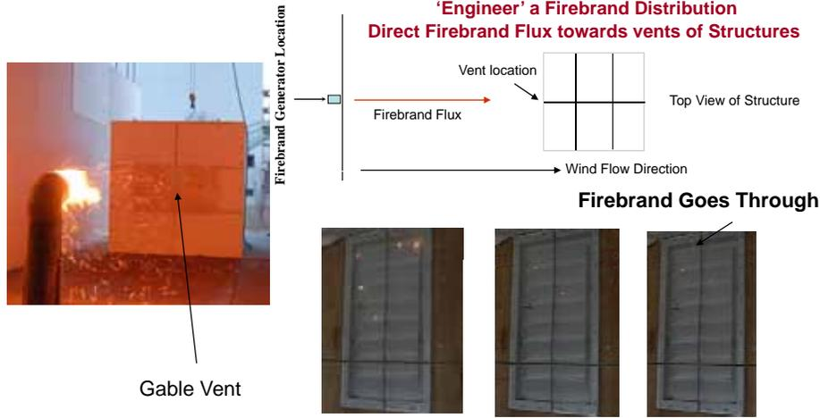
Three sizes tested 6 mm , 3 mm , and 1.5 mm
