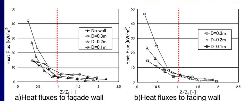
Fig. Heat flux rate to each wall (B0.2 m x H0.2 m)
