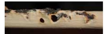
Image of vinyl siding (from bottom) after firebrand exposure at 7 m/s
