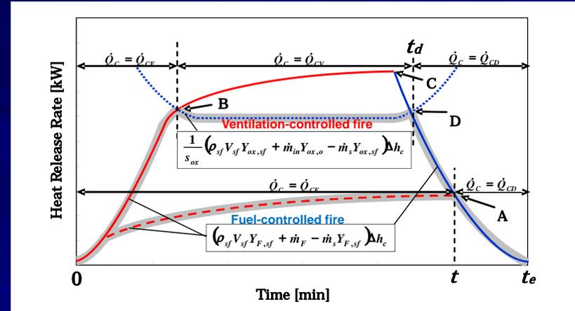
Fig. Transition of heat release rate within a compartment
