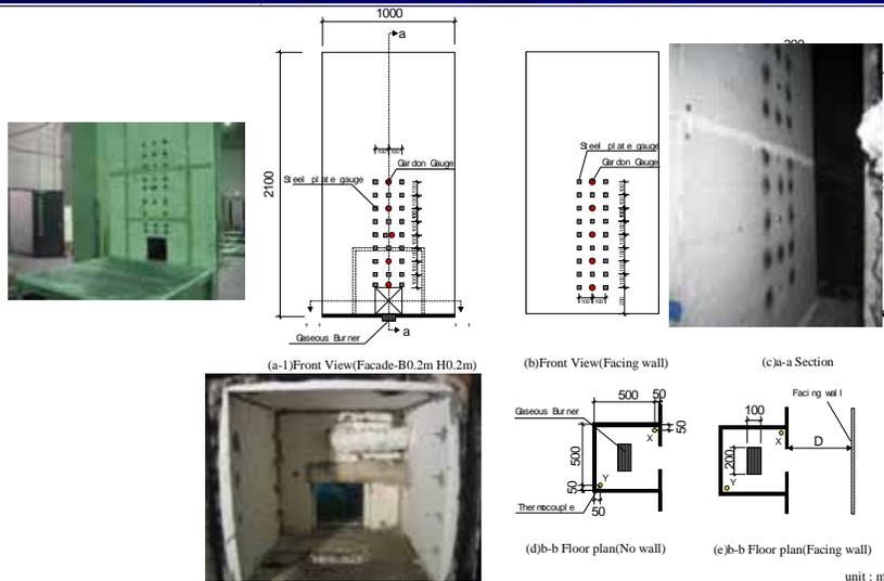
Fig. Experimental setup
