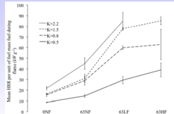
Mean HRR during flaming (global heat of combustion)
