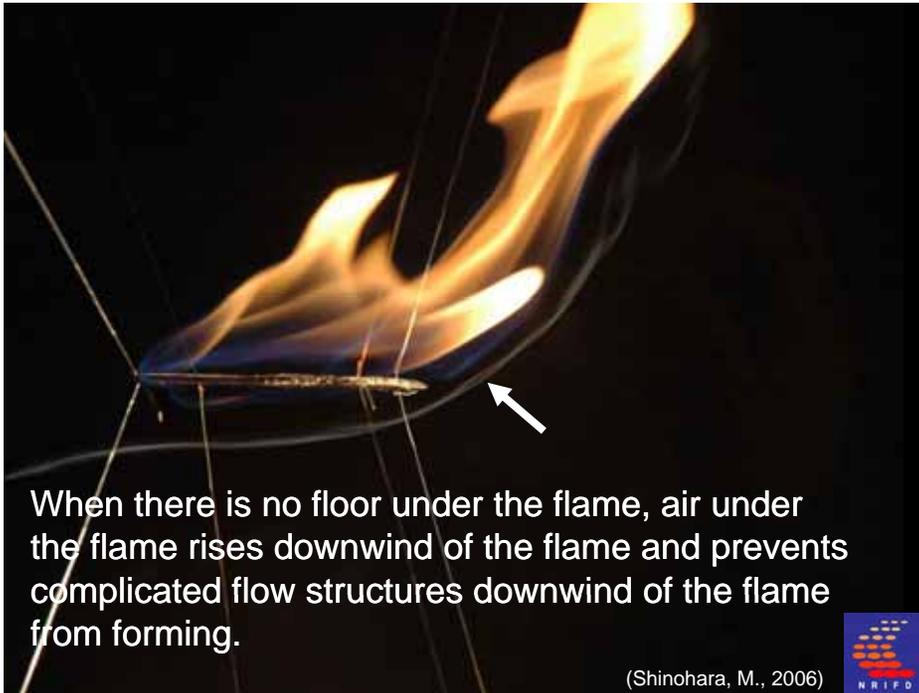
When there is no floor under the flame, air under the flame rises downwind of the flame and prevents complicated flow structures downwind of the flame from forming.
