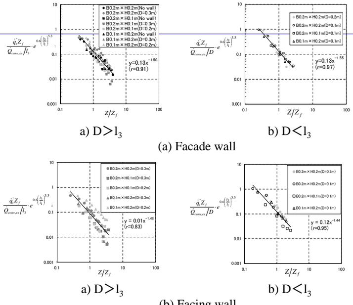
Fig. Non-dimensional height and Non-dimensional heat flux to each wall
