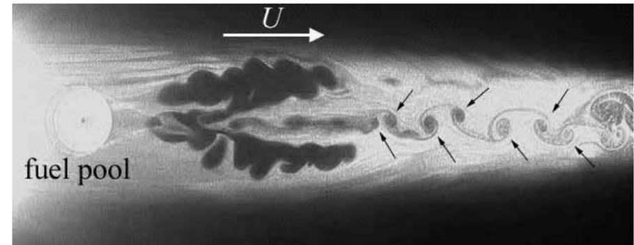
Cross-sectional view  $U = 0.49 \text{ m/s}$   $h_{sw} = 40 \text{ mm}$   $D = 80 \text{ mm}$  Fuel: Methanol
