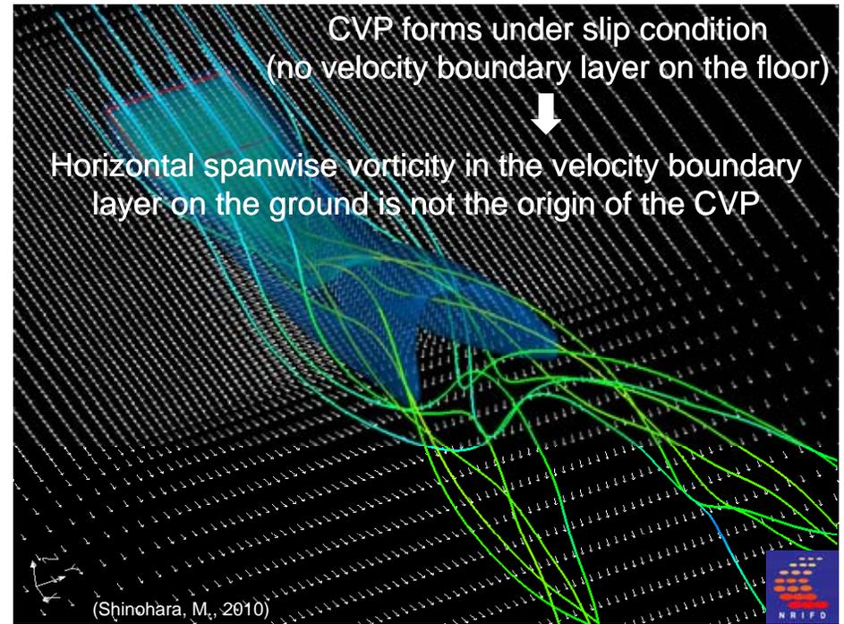
CVP starts from the horizontal **streamwise** vorticity located just above each side edge of the square heated area.
