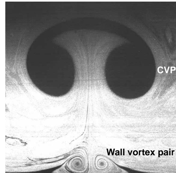
Fuel pool :  $D=3\text{cm}$ ,  $x=18\text{cm}$ ,  $U=0.55\text{m/s}$
