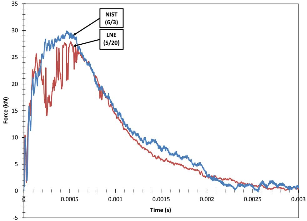
Figure 23 - Selected instrumented curves from 5AB tested at LNE (specimen P33) and NIST (specimen G71).
