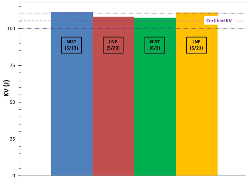
Figure 3 - Average values of absorbed energy KV for HH-103. Dashed line and dotted lines indicate respectively certified value and bounds of  $\pm 5\%$  (acceptability limits according to ASTM E23).
