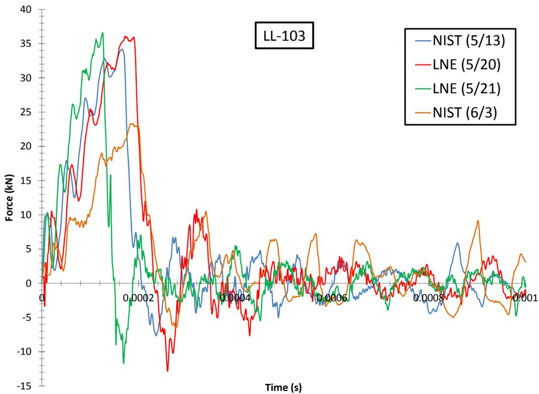
Figure 7 - Comparison between selected LL-103 test records from NIST and LNE testing rounds (NIST, 1<sup>st</sup> round: specimen 938; LNE, 1<sup>st</sup> round: specimen 186; LNE, 2<sup>nd</sup> round: specimen 237; NIST, 2<sup>nd</sup> round: specimen 639).
