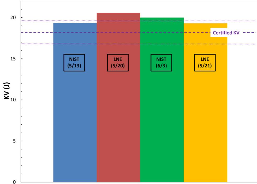
Figure 2 - Average values of absorbed energy KV for LL-103. Dashed line and dotted lines indicate respectively certified value and bounds of  $\pm 1.4$  J (acceptability limits according to ASTM E23).
