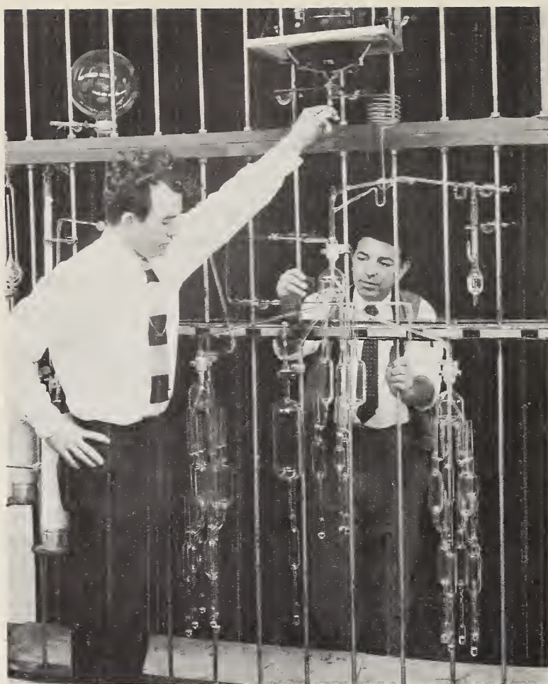
Left: Samples of benzene with controlled amounts of impurity are packaged in a vacuum system. The vacuum transfer system assured the identity of the 42 samples distributed for an international comparison analysis. Right: Analyzing alloys containing minute amounts of titanium, zirconium, niobium, and tantalum. A relatively simple method based on the formation of metal-fluoride complexes was developed for this analysis (pages 51, 49).
