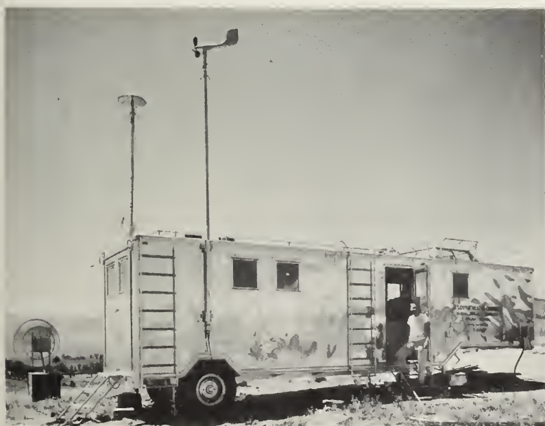
NBS mobile laboratories make it possible to study radio conditions in many parts of the world. At left is a unit at Boulder, Colorado, and at right is a station in North Africa (page 116).
