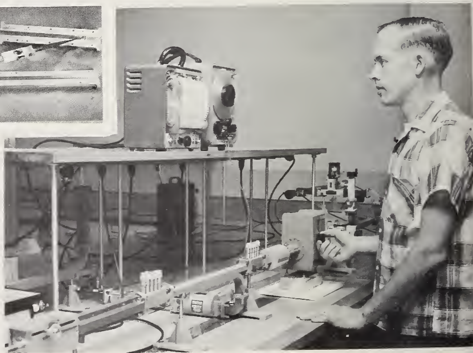
The half-round obstacle-type microwave impedance standard above is the heart of a new technique for measuring microwave impedance (page 124).
