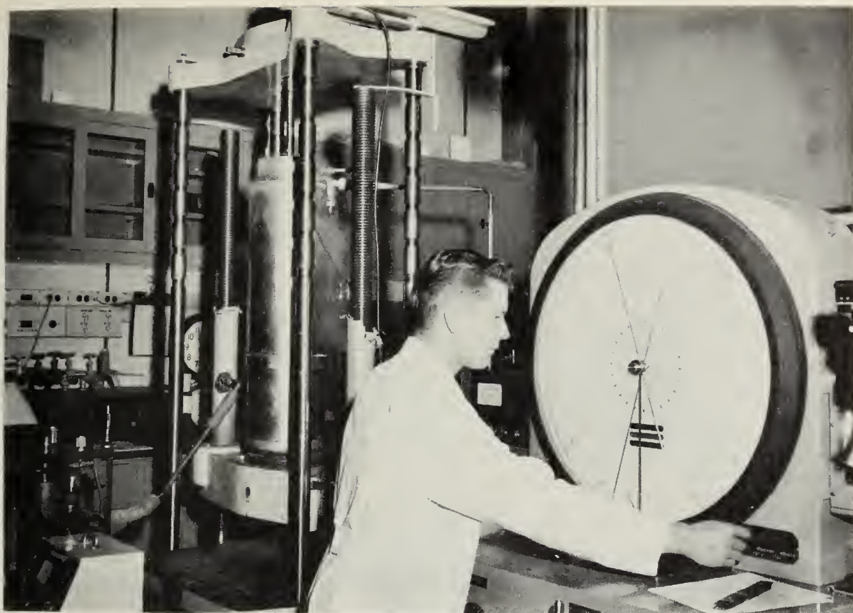
Low-temperature data on the compression deformation of indium were obtained prior to its use to seal the massive glass window of the 72-inch liquid hydrogen bubble chamber for the University of California (page 105).
