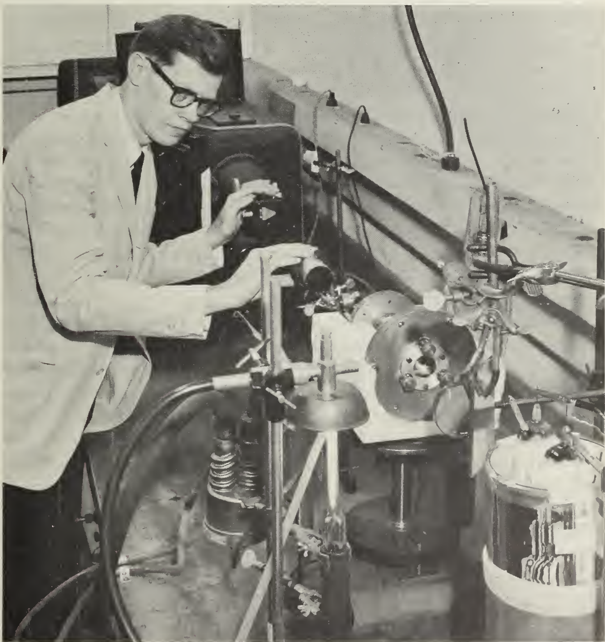
Equipment used in the redetermination of the Rydberg constant. As a result of this work, it is now the most accurately known atomic constant. The work was done as part of a program of obtaining more accurate values for important physical constants (pages 3, 29).
