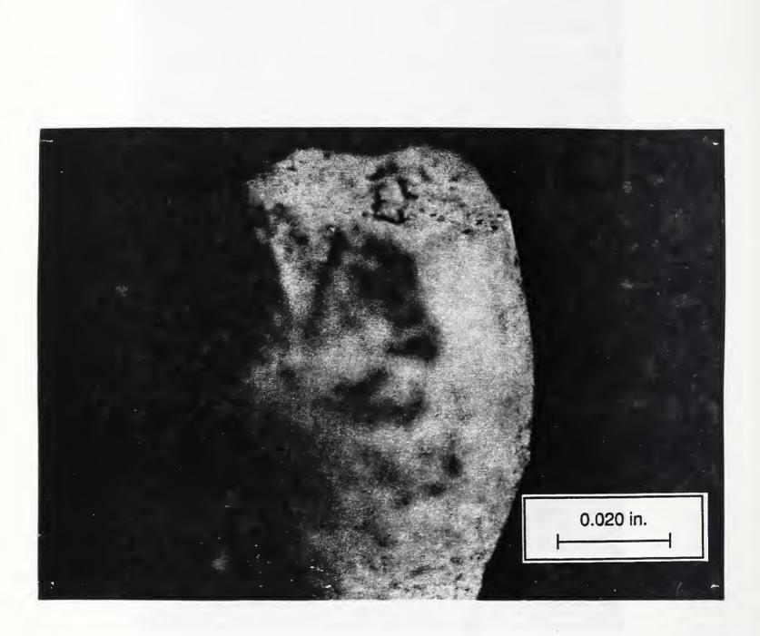
Figure 8. Specimen 2, Sand Grains Adhered to Upper Wire,  $0^{\circ}$ -Viewing Angle.
