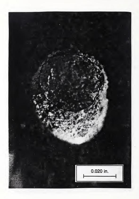
Figure 12. Specimen 3, Sand Grain Adhered to Upper Wire, Estimated Planar Bond Failure Surface Area (Used in Table 1) Shown by Enclosed Area, 90°-Viewing Angle.
