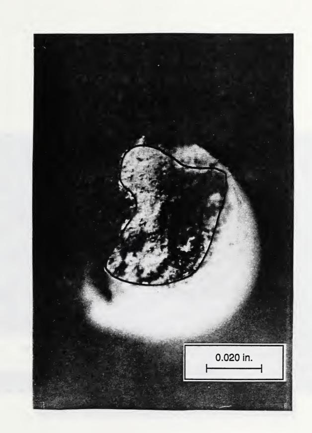
Figure 7. Specimen 2, Sand Grain Adhered to Upper Wire, Estimated Planar Bond Failure Surface Area (Used in Table 1) Shown by Enclosed Area, 90°-Viewing Angle. See Footnote "d" in Table 1.
