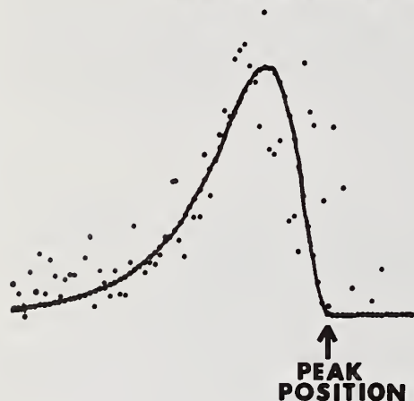
Figure 6. The iron Kα incomplete charge residuals remaining after subtracting a fitted Gaussian curve from a real peak. The smooth points are a fit to the residuals using equation 6.
