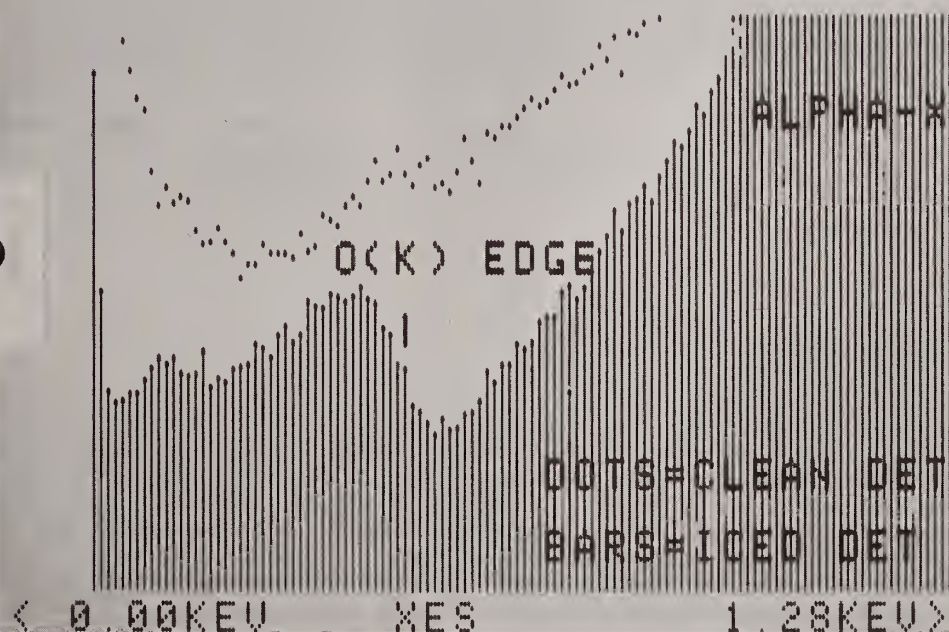
Figure 5. Comparison of the beta-induced x-ray spectrum of a ErDT film on molybdenum for a Si(Li) detector iced and clean. The spectra were normalized at the large Er(M) peak. (a) 0 - 2.56 keV and (b) 0 - 1.28 keV.
