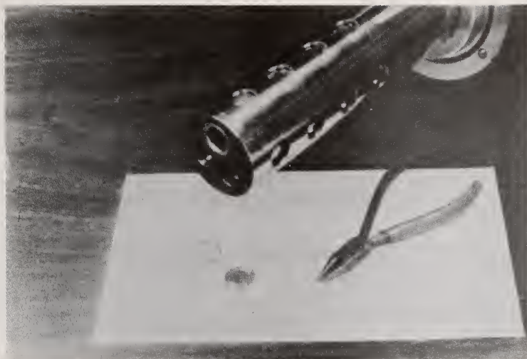
Figure 3. Organic window mounted on an aluminum ring, held in place with an easily removed c-clip.
