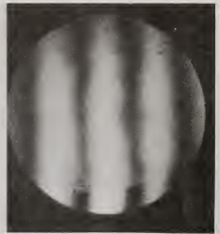
2 HOURS AFTER 50°C OVEN FRINGES VERTICAL
