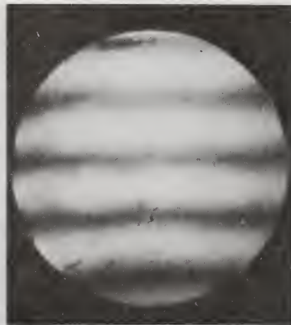
3 HOURS AFTER 100°C OVEN FRINGES HORIZONTAL
