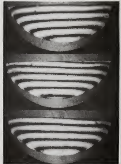
Figure 6. Interference fringes showing initial distortion and ultimate optical figure error of a ULE flat after thermal cycling to various temperatures up to 350°C. Both an air quench and a water quench were used. No ultimate thermally induced figure error can be observed for this material.
