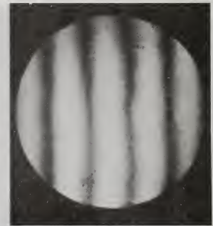
3 HOURS AFTER 150°C OVEN FRINGES VERTICAL
