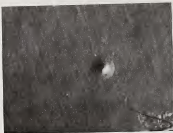
Figure 5. Laser damage at 1.06 μm on same surface shown in figure 4 after heat treatment. Note the marked change in damage morphology.
