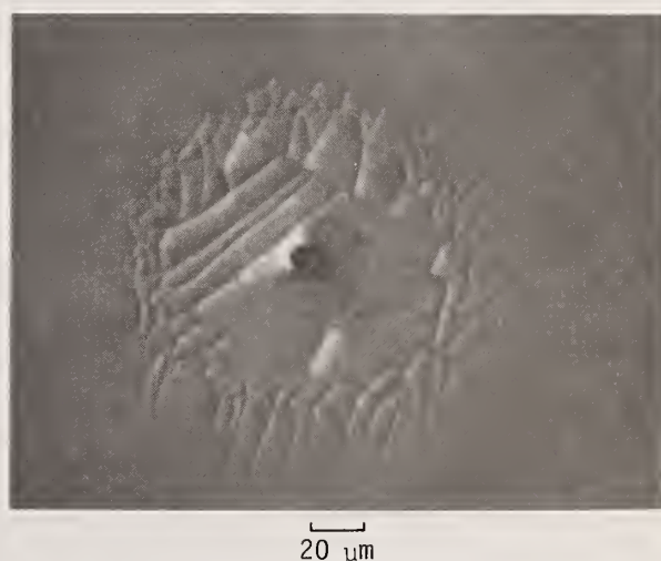
Figure 4. Laser damage at 1.06 μm on a polished, untreated NaCl surface.
