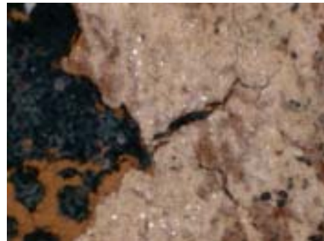
1000 °C for an hour massive spalling of paint, falls off thick scale forms between paint and steel
