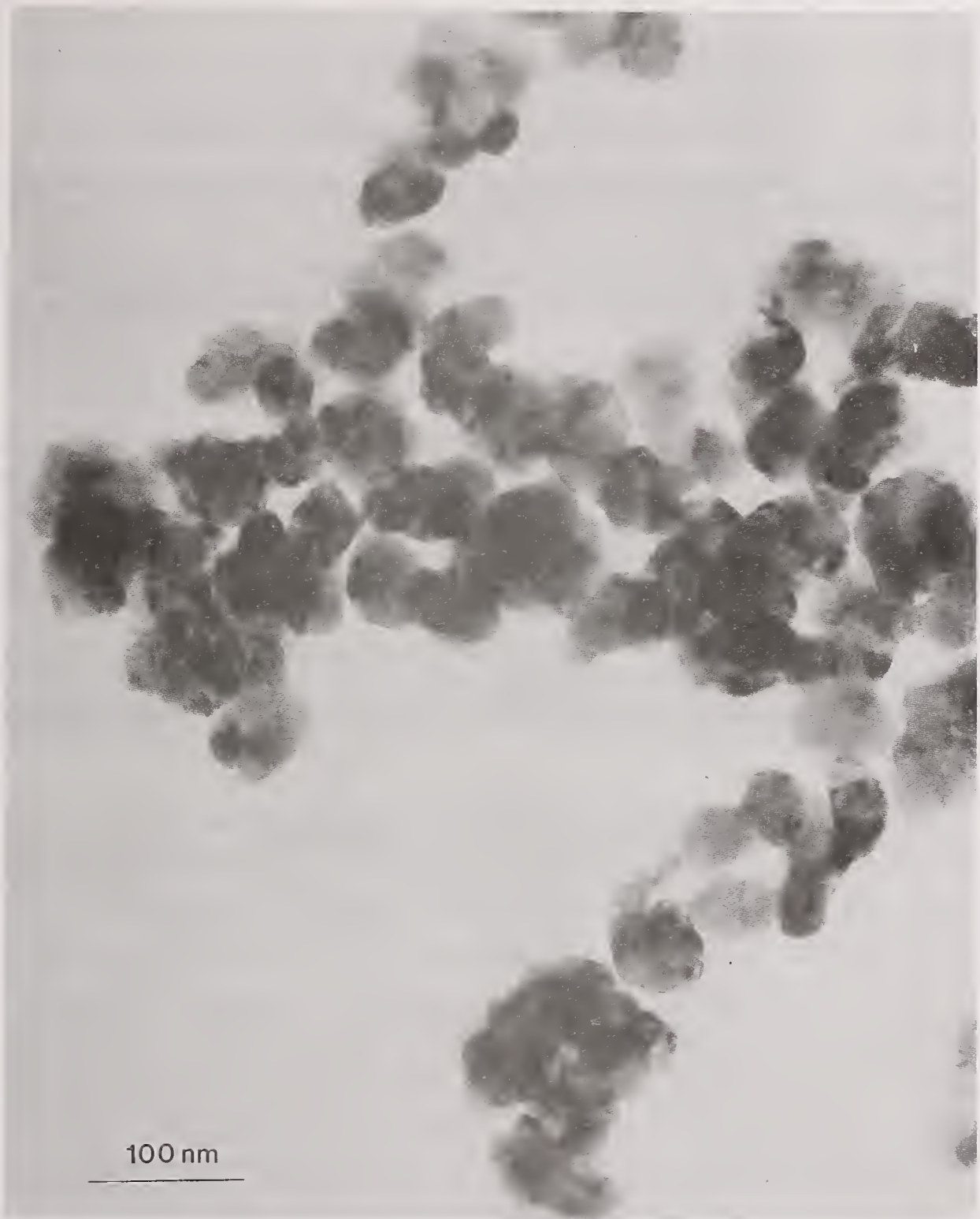
Figure 66. TEM micrograph of primary particles. Sample: YSZ 0269. Lab No. 22.
