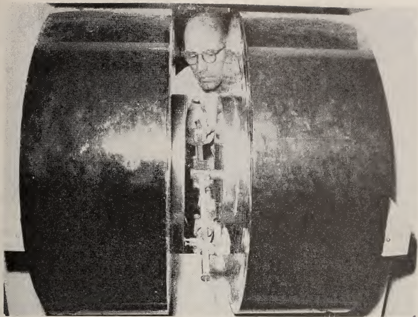
A ferrite rod mounted in a cylindrical cavity is placed between the poles of an electromagnet. The microwave electrical constants of ferrites are accurately measured with this equipment (p. 92).
