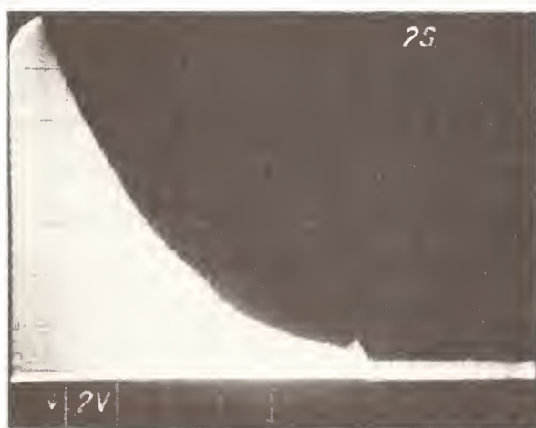
Fig. 2 Measured backscattered level from a 10 km long fiber
