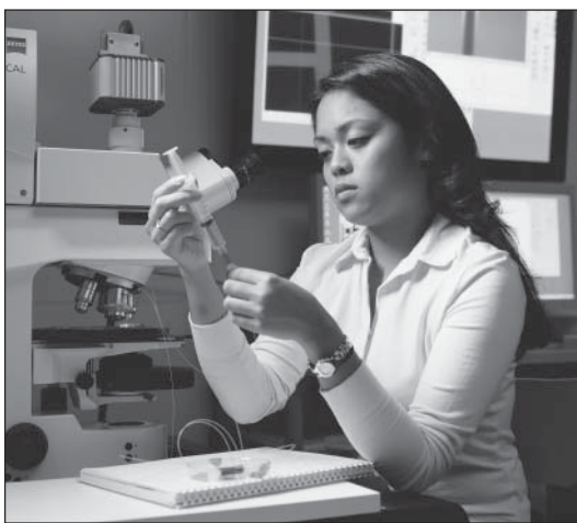
Geraldine Mijares using a confocal fluorescence imaging microscope to characterize microfluidic systems prepared with microelectrodes. Copyright Robert Rathe
