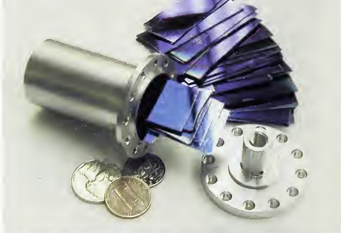
FIGURE 1. A stack of 1014 Å PC films (notice the blue tint) on thin slabs of Si ready to go into the HFBS spectrometer.
