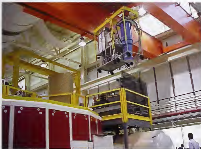
FIGURE 6. Superconducting magnet/dilution refrigerator as it is being lifted onto the DCS spectrometer. The adjustable lifting frame compensates for the lifting point shifting in case liquid cryogenes are added.
