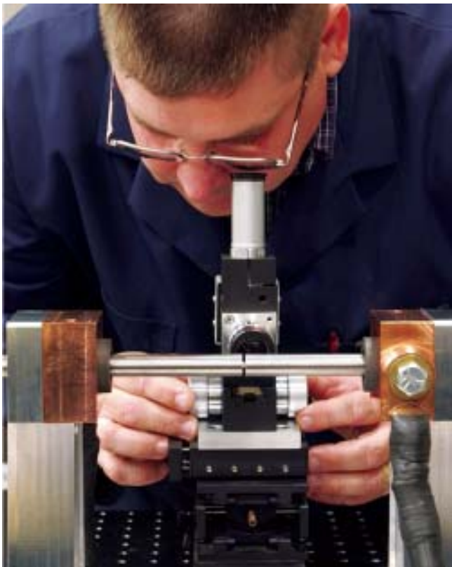
Figure 2: The current for heating is introduced through copper blocks and graphite bearings to the incident and transmitted bars, and then through the sample seen in the middle. The sample temperature is monitored by the pyrometer being focused on it.
